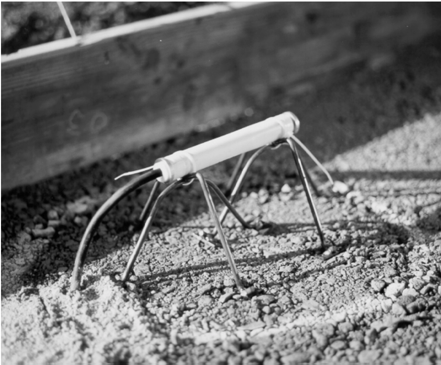
Figure 21a. Carlson A-8 strain meter on its cradle to maintain gage height and
