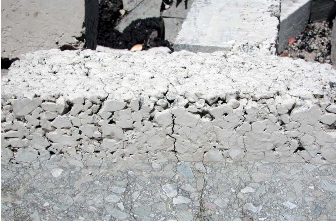
Figure 40a. Fines-clogged ATPB slab from Section 543.
