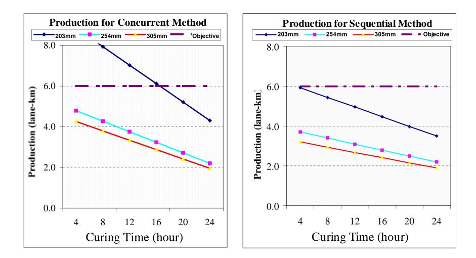
Figure 15. Double-lane production capability (lane-km) graphs.
