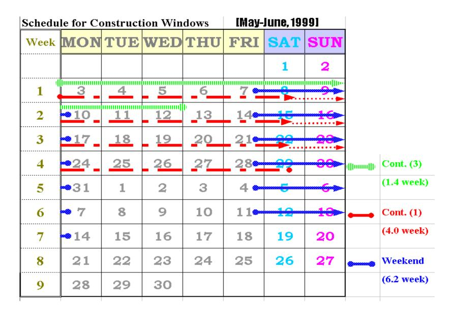
Figure 21. Example of scheduling for different construction windows.
