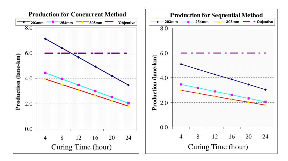
Figure 14. Single-lane production capability (lane-km) graphs.
