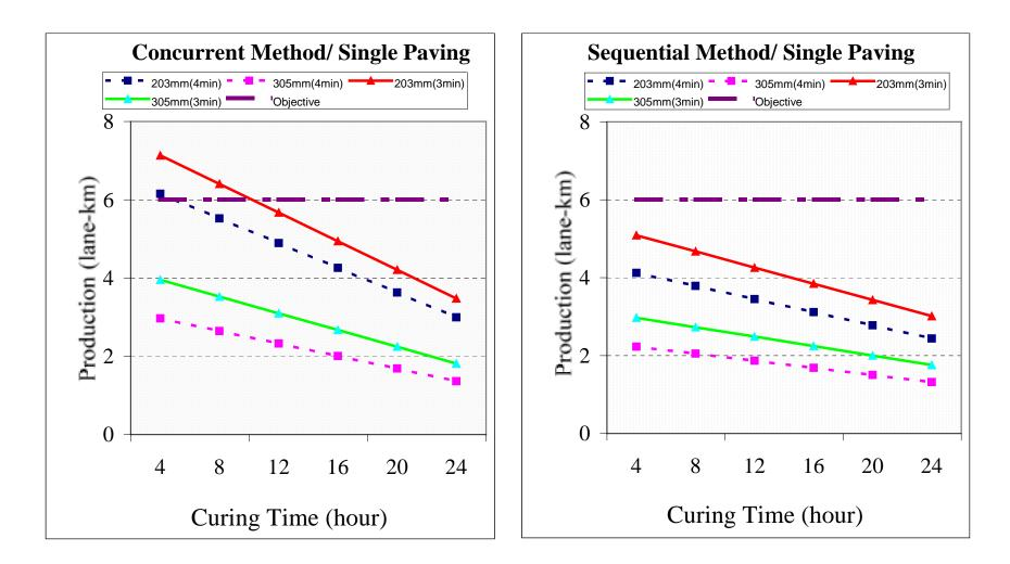
Figure 17. Reduction of production capability (lane-km) by changing the number of trucks from 20 (Cycle=3 min.) to 15 (Cycle=4 min.) per hour.
