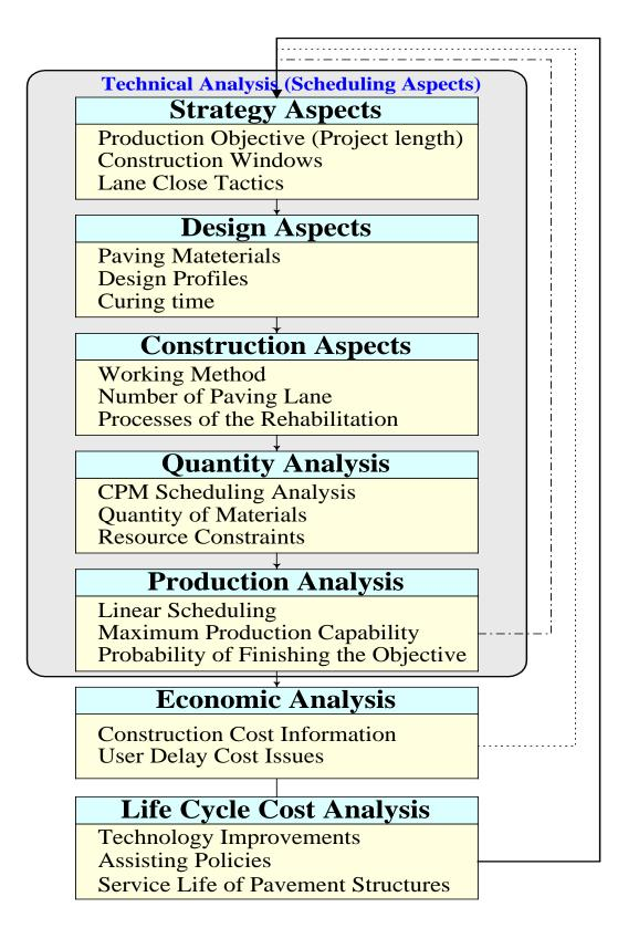
Figure 8. Process of the constructability analysis.
