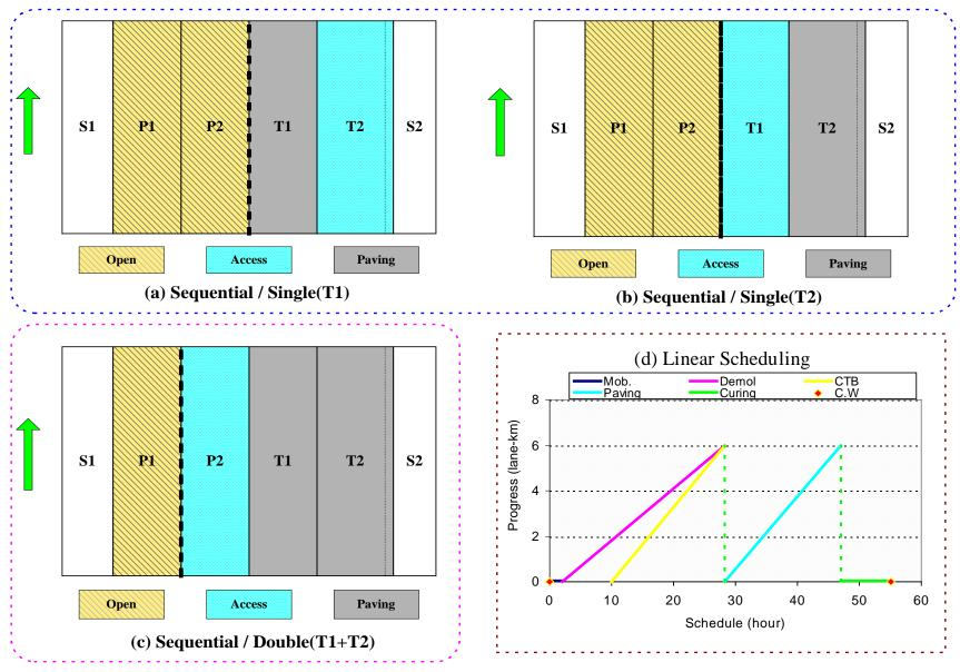
Figure 7. Work plan for sequential working method.
