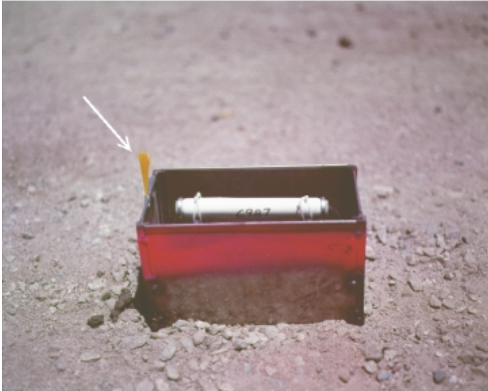
Figure 6.8. Instrument Box with Turkey Tail Attached.
