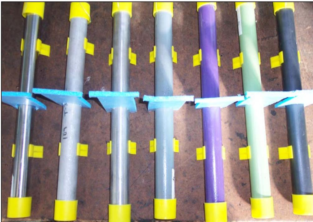
**Figure 6. Different types of steel dowels investigated. From left to right: microcomposite steel, stainless steel hollow, stainless steel-clad, non-bendable epoxy-coated dowel (gray coating), non-flexible epoxy-coated dowel (purple coating), flexible epoxy-coated dowel (green coating), carbon steel.**
