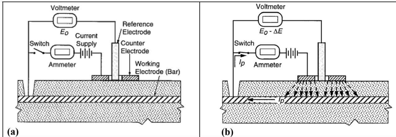
**Figure A2. Three-electrode Linear Polarization Resistance method. (a) Measurement of the open-circuit potential (half-cell potential); (b) Current applied to the counter electrode to produce a small change in voltage  $E_0 - \Delta E$ .**
