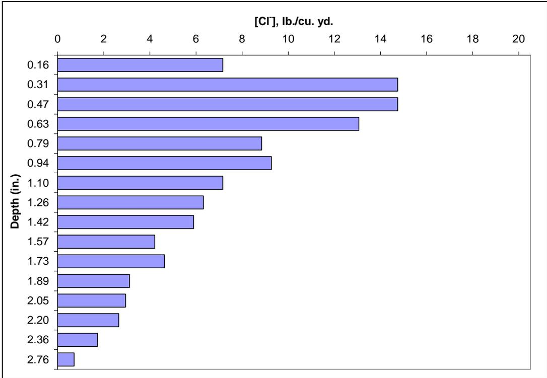
Figure 56. Chloride profile of the slab concrete (Core #1).
