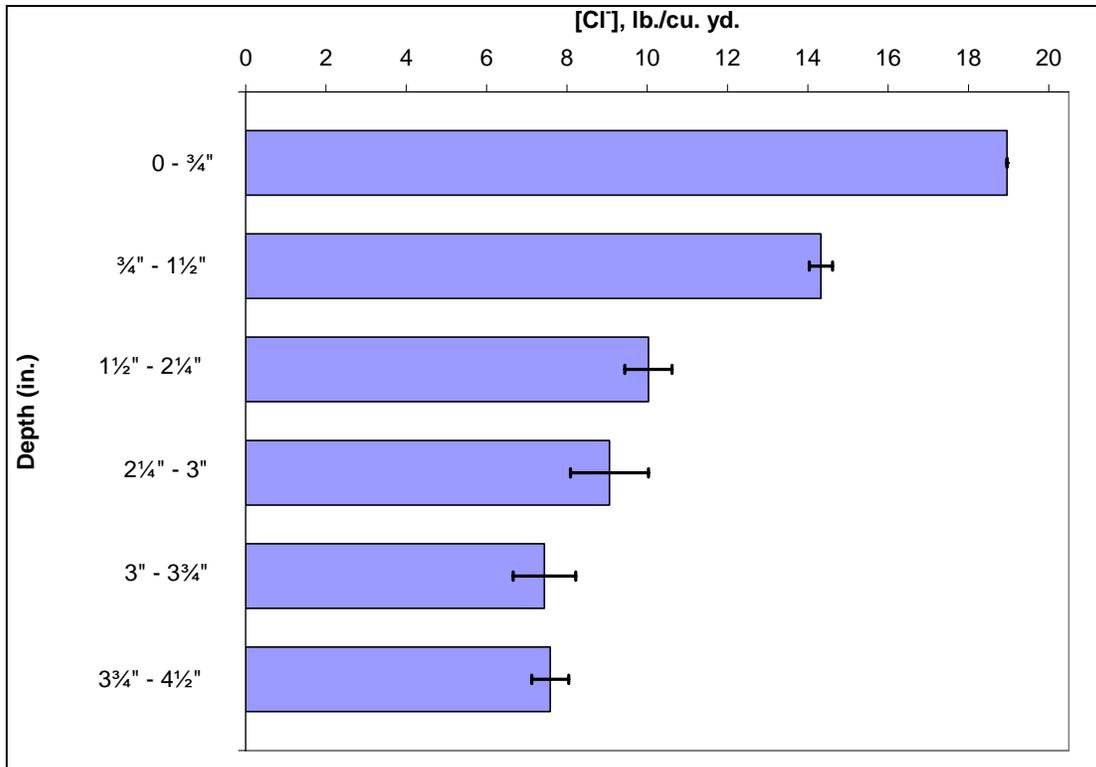
Figure 63. Chloride profile for I- 90 MP 61.304 (Price Creek).
