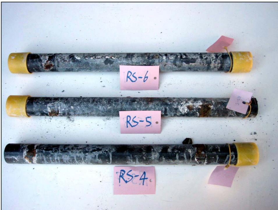
**Figure 22. Corrosion along the carbon steel bars.**
