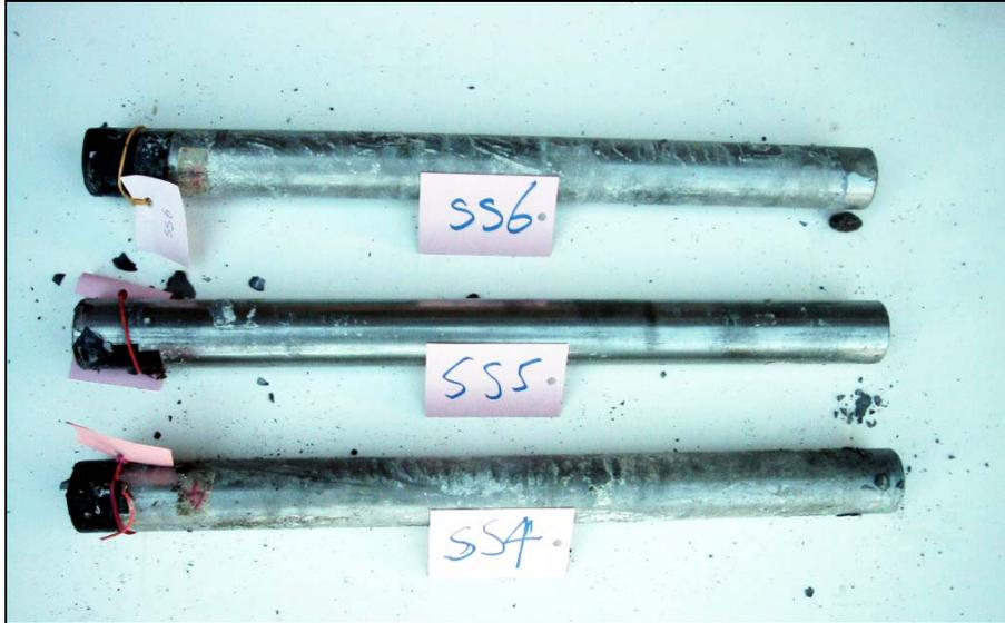
Figure 24. Appearance of stainless steel hollow bars after tests.
