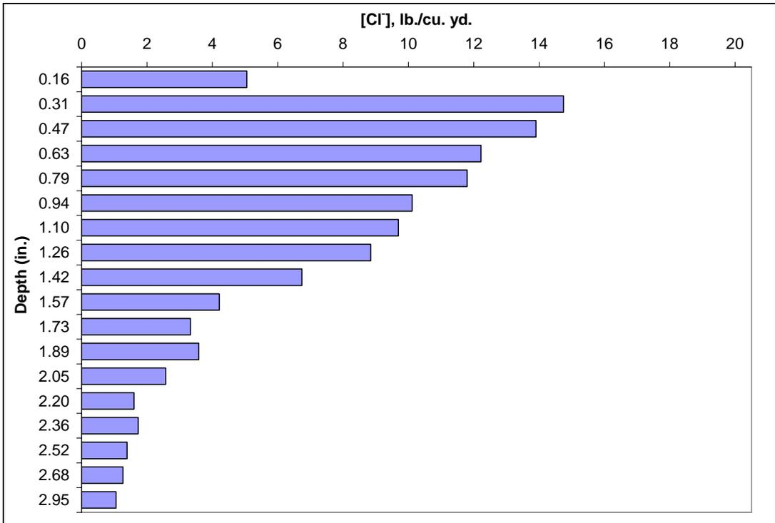
Figure 57. Chloride profile of the slab concrete (Core #2).
