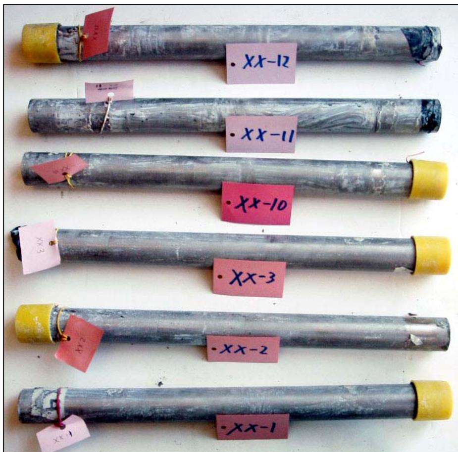
Figure 25. Appearance of stainless clad bars after tests.
