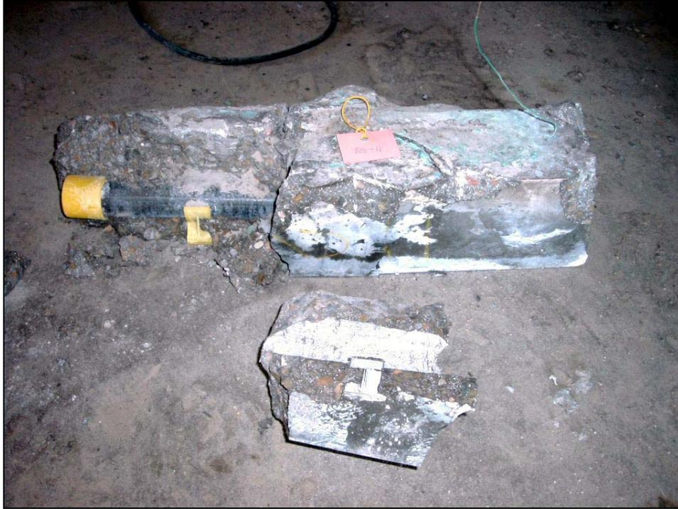
Figure 21. Extraction of dowels for visual inspection.
