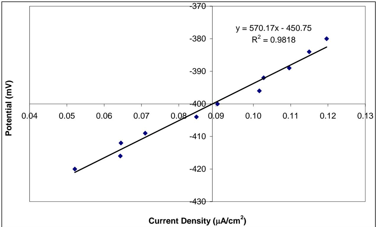
Figure 52. Linear Polarization Resistance, WSDOT slab, Specimen B.
