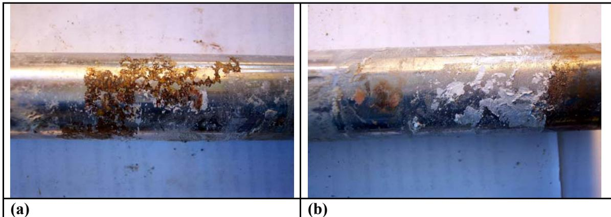
**Figure 37. Microcomposite steel dowels. (a) General view of the center region below joint; (b) End region.**
