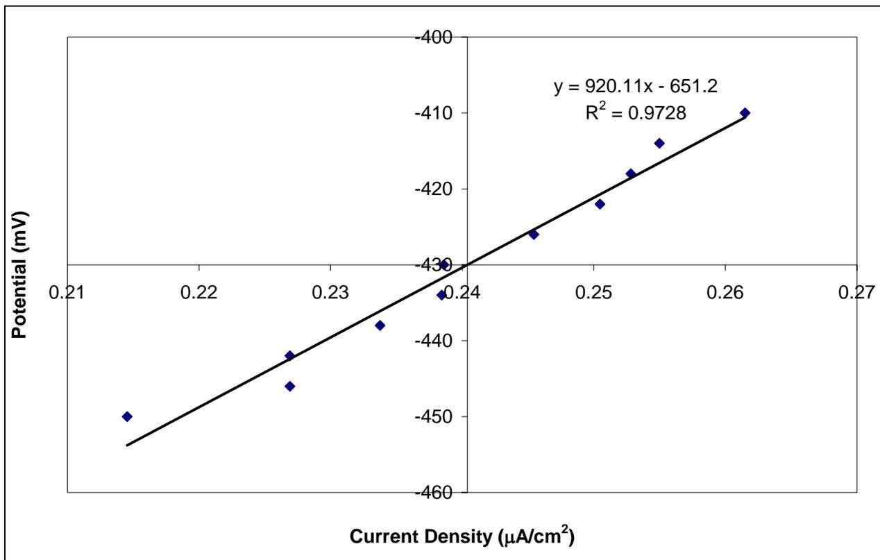
Figure 51. Linear Polarization Resistance, WSDOT slab, Specimen A.
