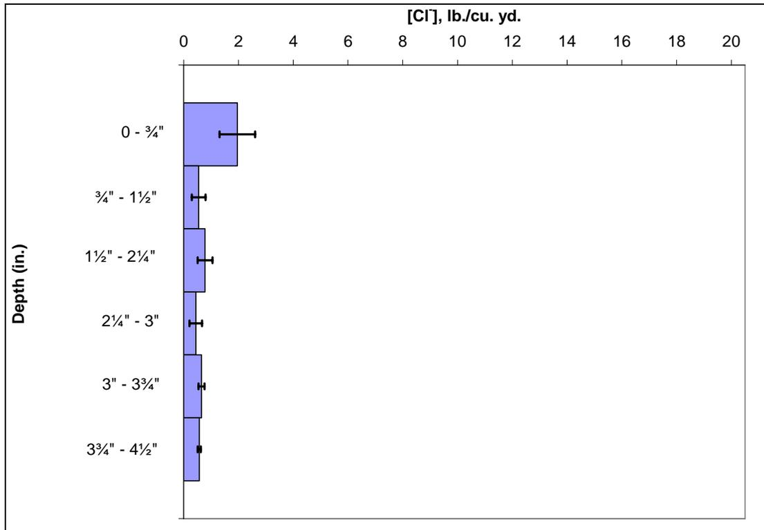
**Figure 65. Chloride profile for SR 82 MP 43.524 (Wapato).**
