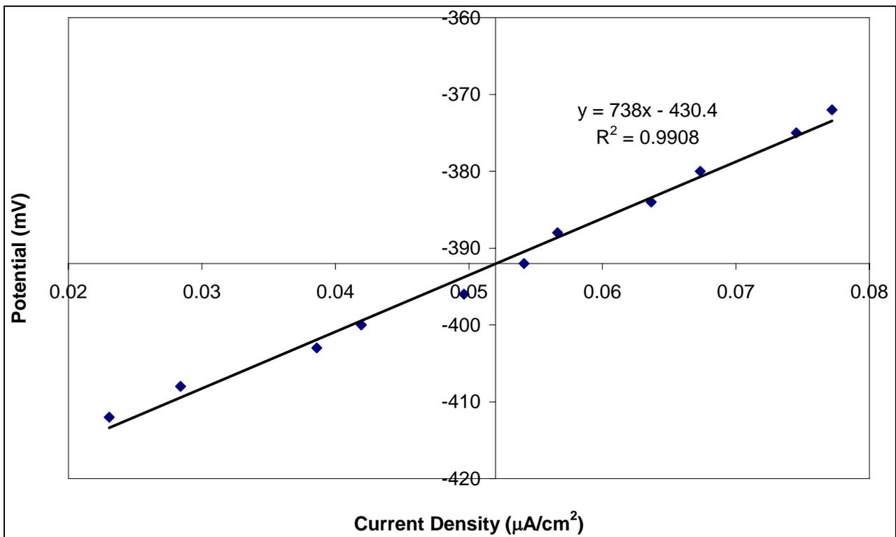
Figure 53. Linear Polarization Resistance, WSDOT slab, Specimen C.
