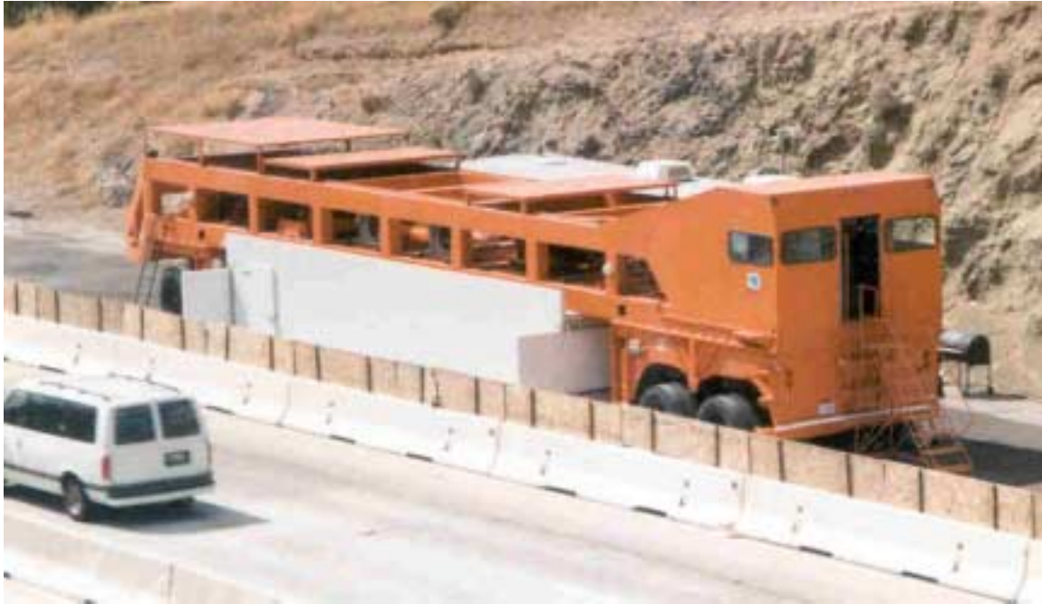
Figure 1.1. HVS with temperature control chamber at the Palmdale test sections.
