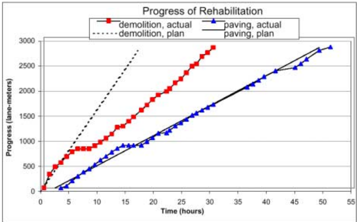
Figure 62. Actual progress of the rehabilitation compared with planned progress.
