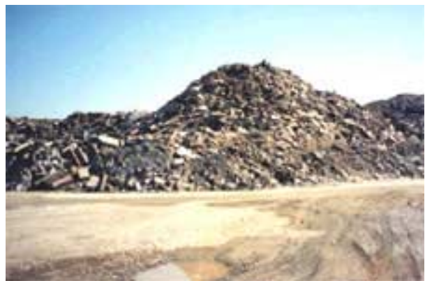
Figure 27. Stockpile of rubblized concrete.
