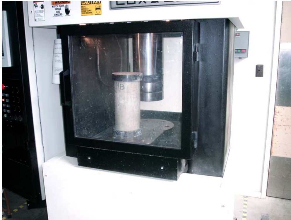
Figure 2.5. Compressive strength test configuration.
