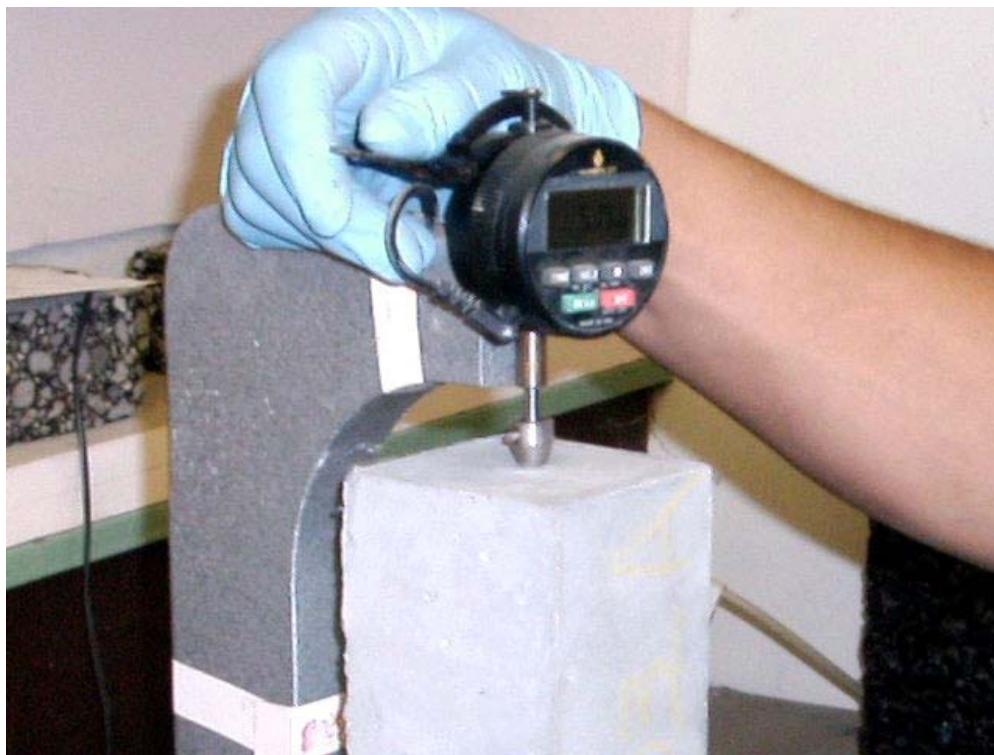
Figure 2.6. Shrinkage test configuration.
