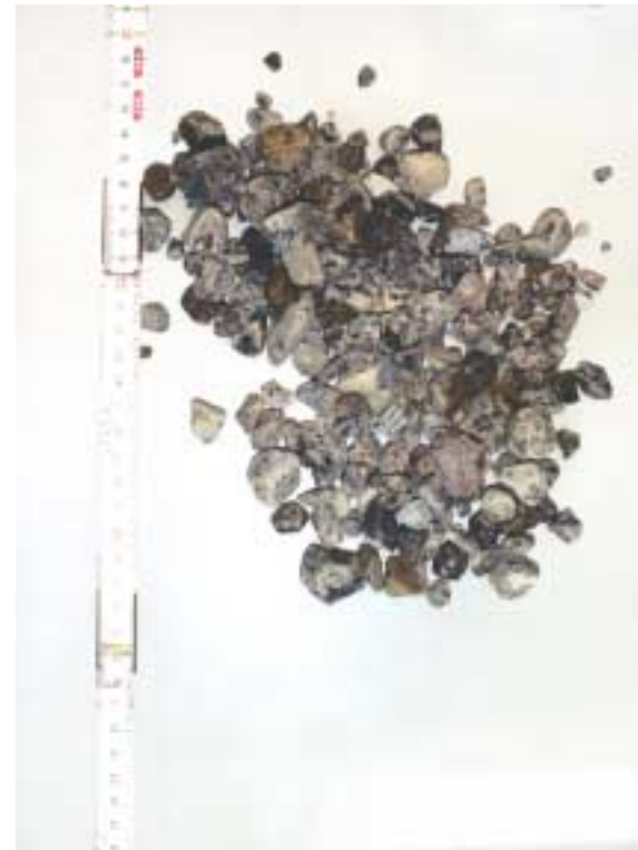
b. Asphalt Treated Permeable Base
