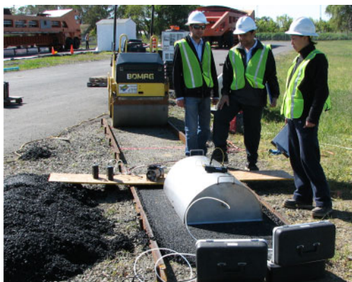
Figure 9. Portable flux chamber for measuring emissions during paving.
