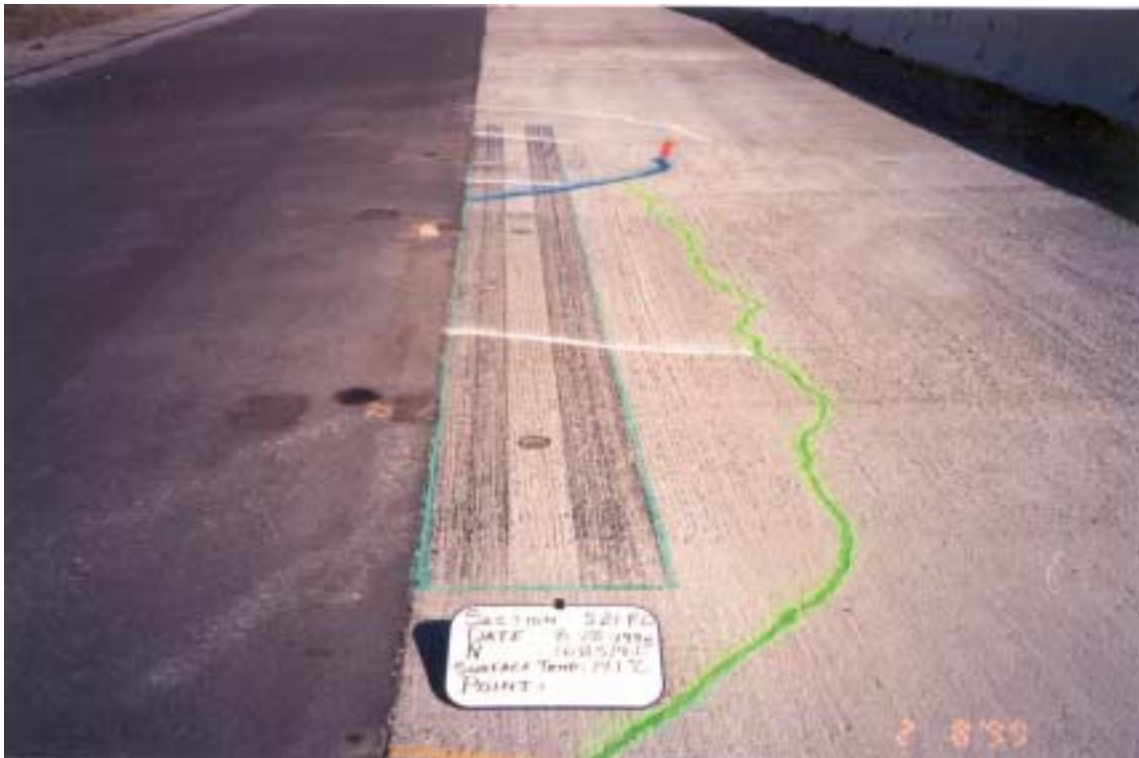
Photograph 4.17. Final Crack pattern after 168,319 repetitions, Test Section 521FD.
