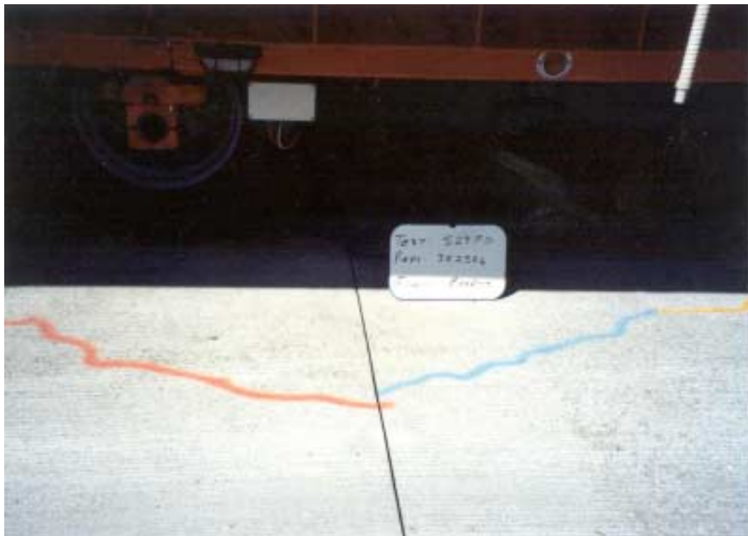
Photograph 4.38. Final crack pattern after 352,324 repetitions, Test Section 529FD.
