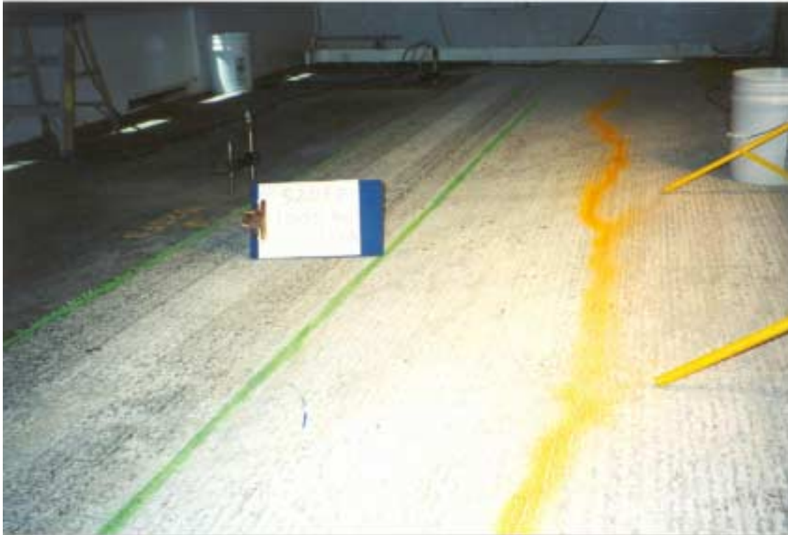
Photograph 4.9. Longitudinal crack after 1,000 repetitions, Test Section 520FD.
