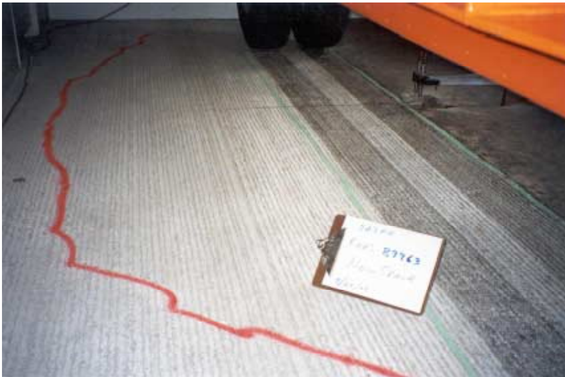
Photograph 4.23. Crack pattern after 90,000 repetitions, Test Section 523FD.
