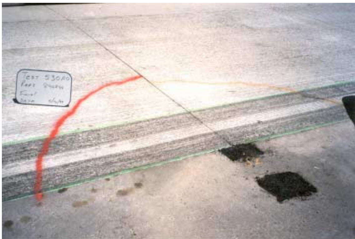
Photograph 4.40. Final crack pattern at the end of the test (846,844 repetitions), Test Section 530FD.
