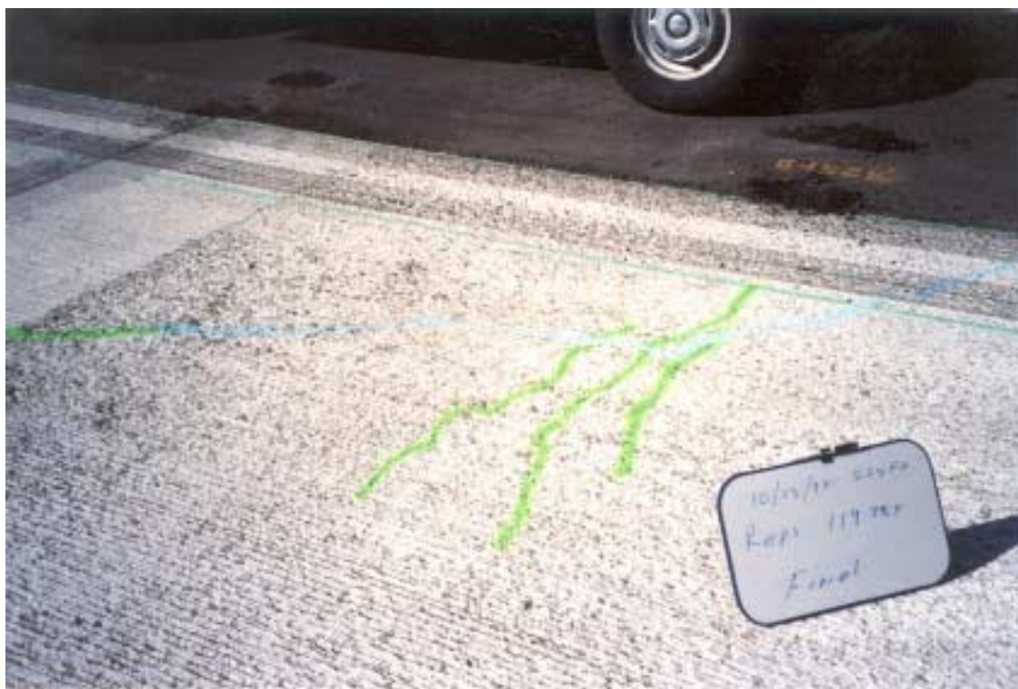
Photograph 4.25. Crack pattern at completion of HVS trafficking, Test Section 524FD.
