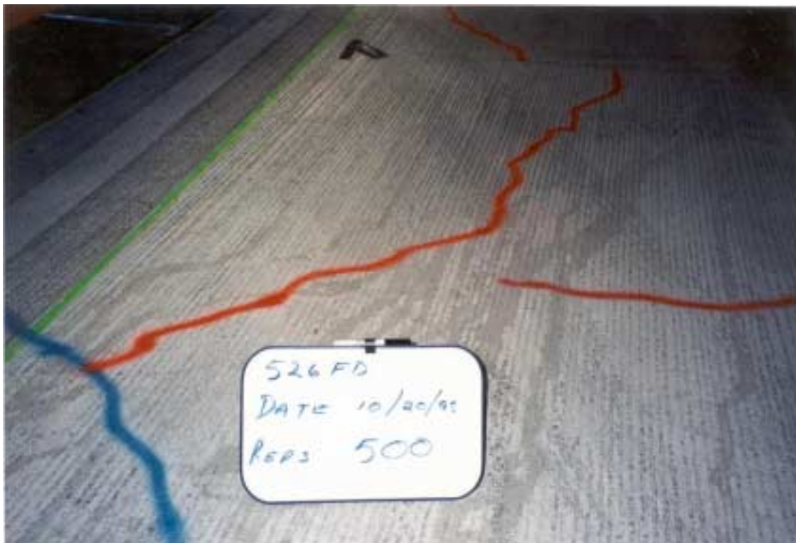
Photograph 4.29. Crack pattern after 500 repetitions, Test Section 526FD.
