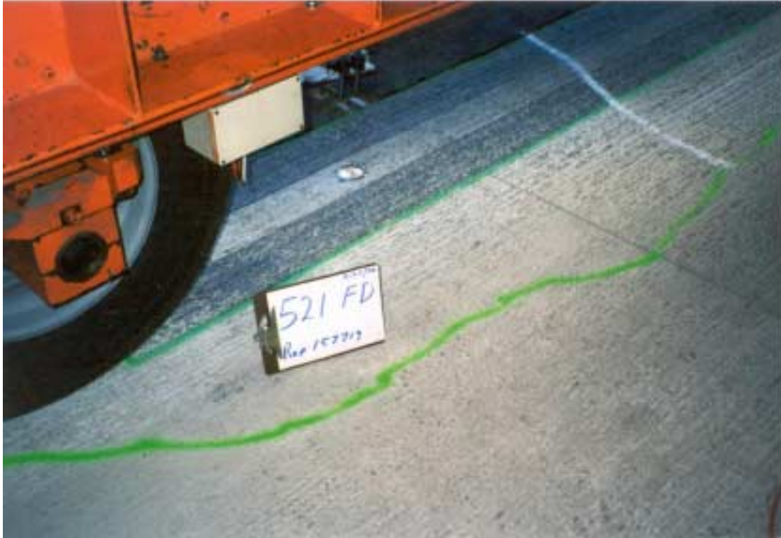
Photograph 4.16. Corner cracks at joint after 157,000 repetitions, Test Section 521FD.
