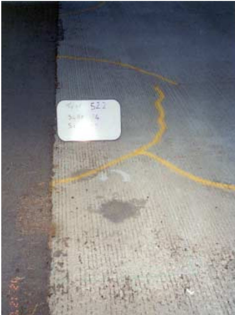
Photograph 4.19. Crack pattern prior to HVS testing, Test Section 522FD.
