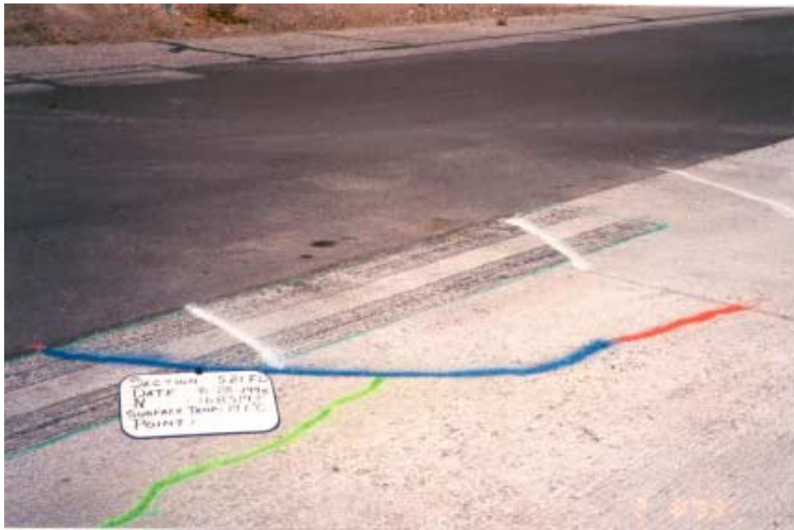
Photograph 4.15. Crack pattern after 168,000 repetitions, Test Section 521FD.
