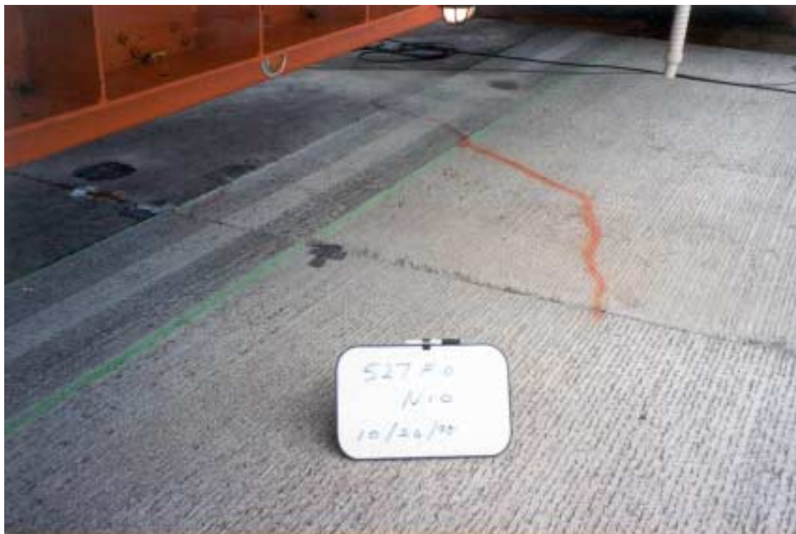
Photograph 4.32. Corner crack at start of test, Test Section 527FD.
