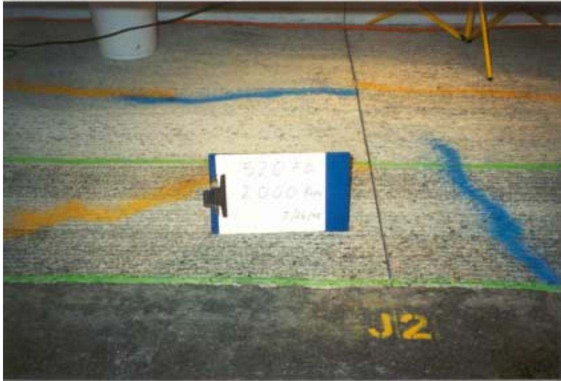
Photograph 4.10. Cracks at joint 7 (J2) after 2,000 repetitions, Test Section 520FD.
