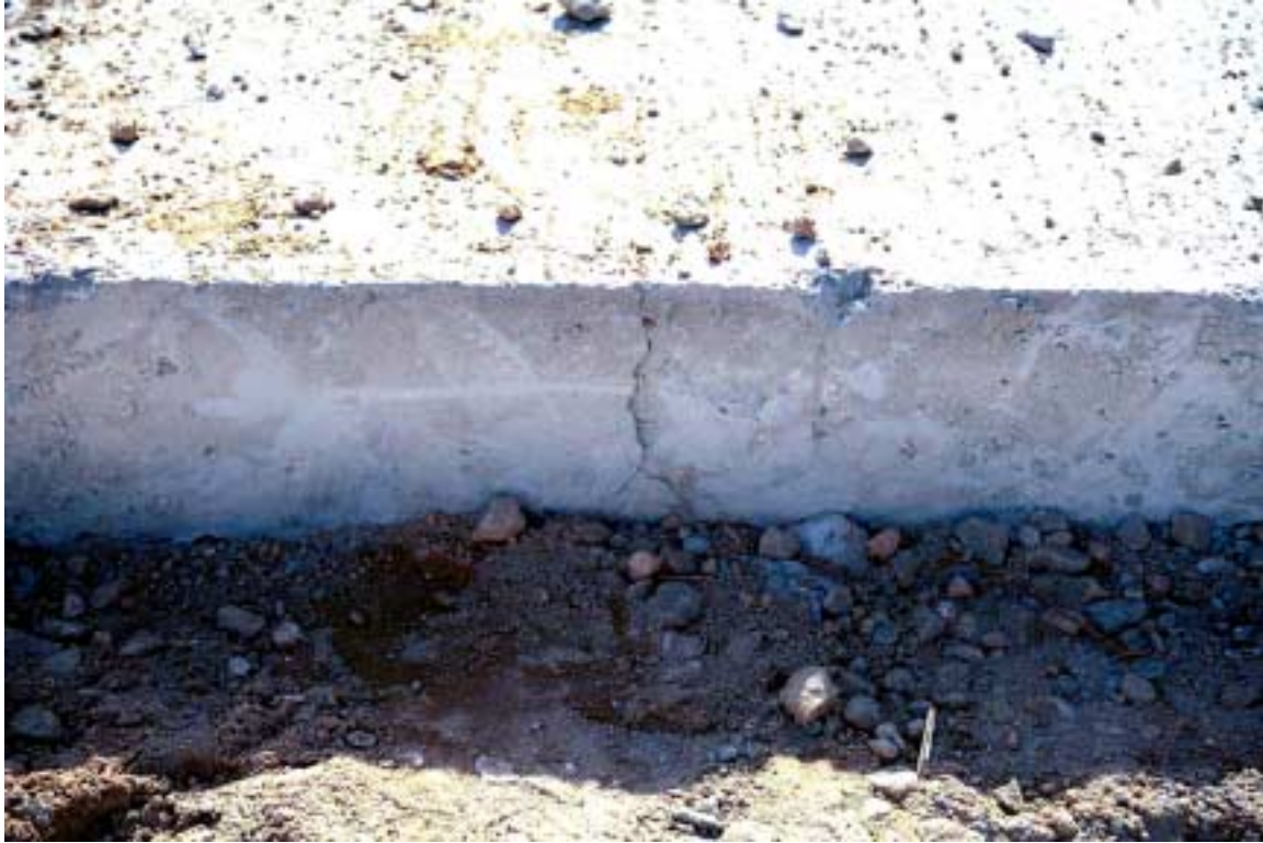
Photograph 5.3. Crack on Test Section 525FD.
