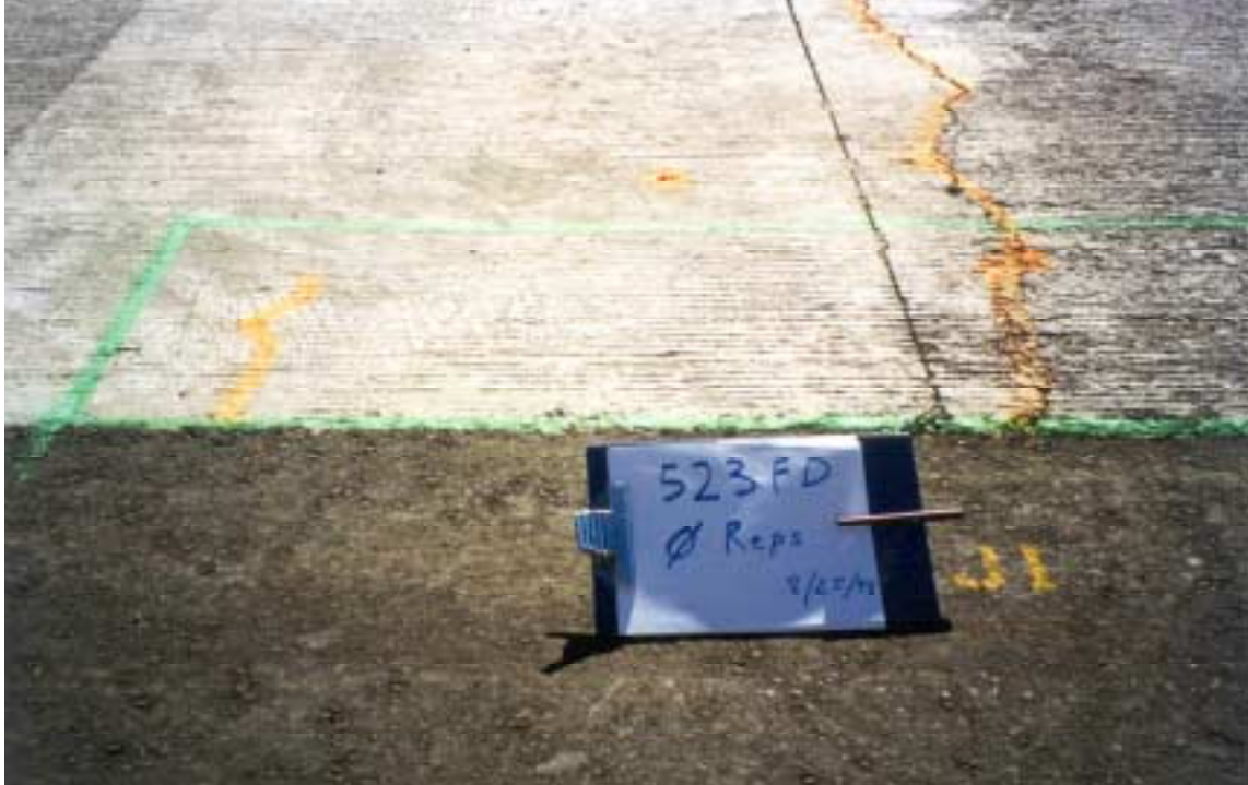
Photograph 4.22. Crack at transverse joint (joint 17) at start of test, Test Section 523FD.
