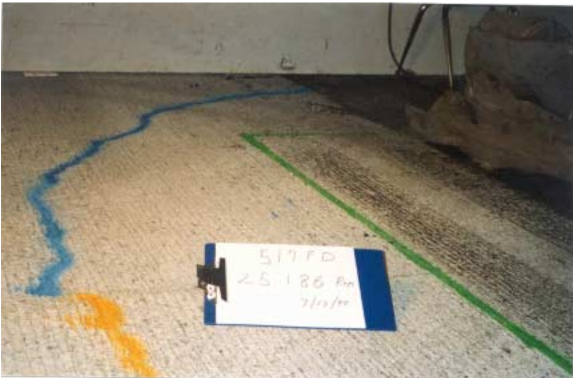
Photograph 4.4. Corner crack on slab 3 25,000 repetitions, Test Section 519FD.
