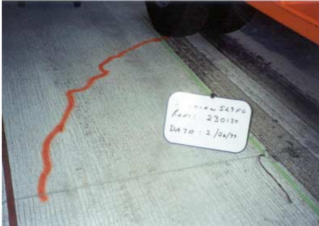
Photograph 4.37. Corner crack after 230,000 repetitions, Test Section 529FD.
