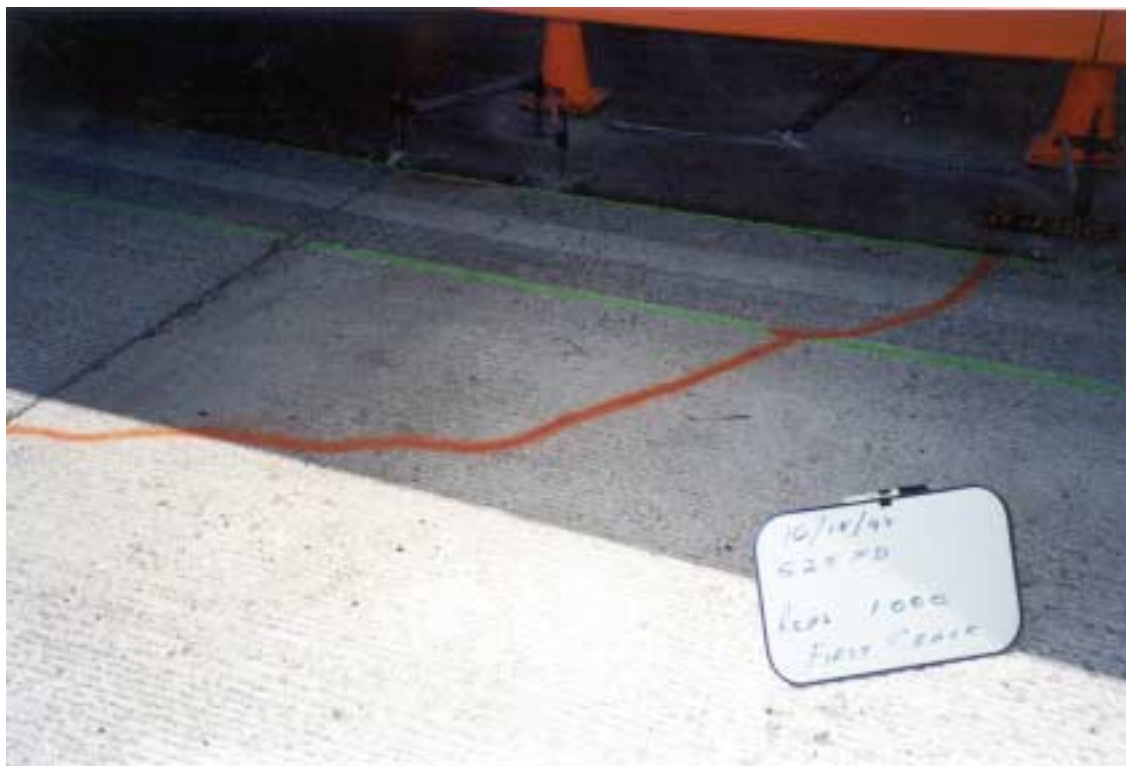
Photograph 4.27. Corner crack after 1,000 repetitions, Test Section 525FD.
