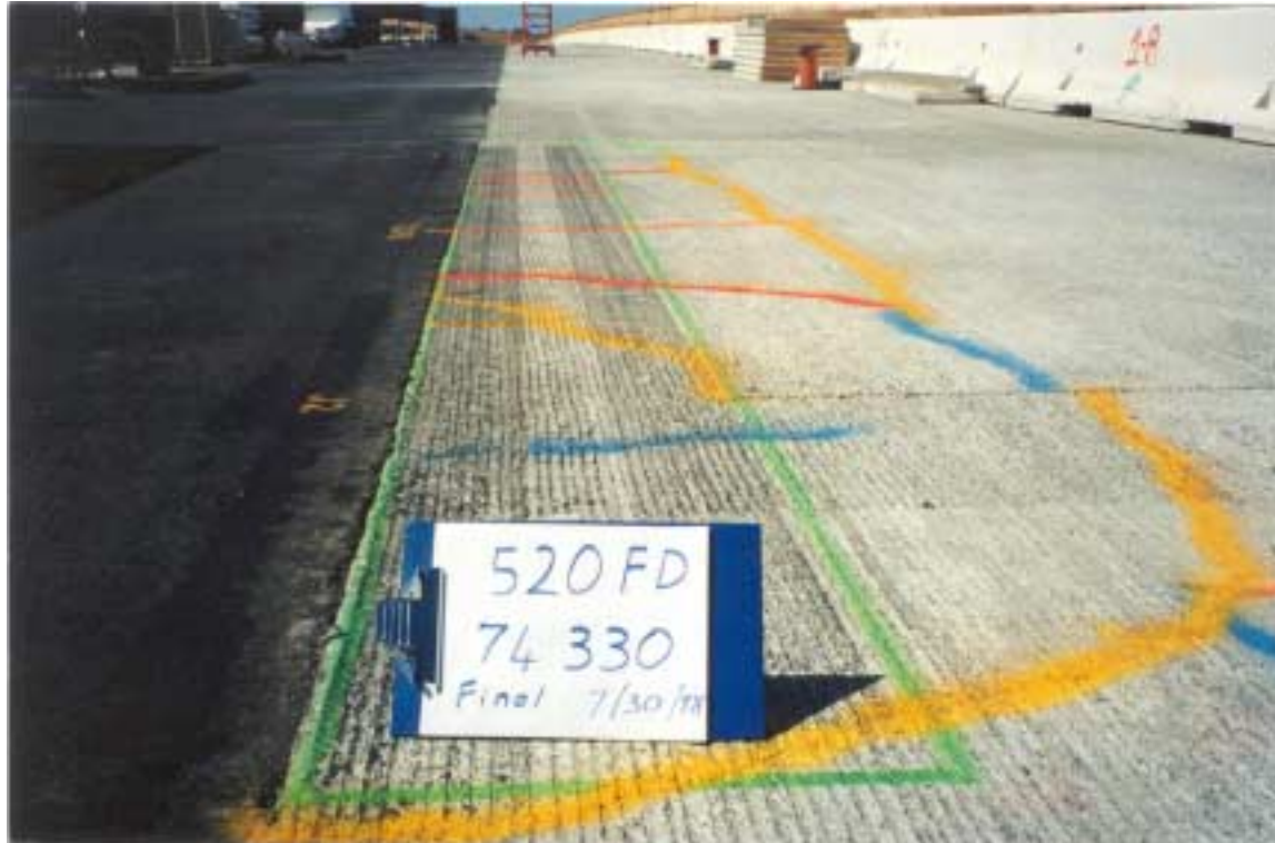
Photograph 4.11. Final crack pattern after 74,000 repetitions, Test Section 520FD.
