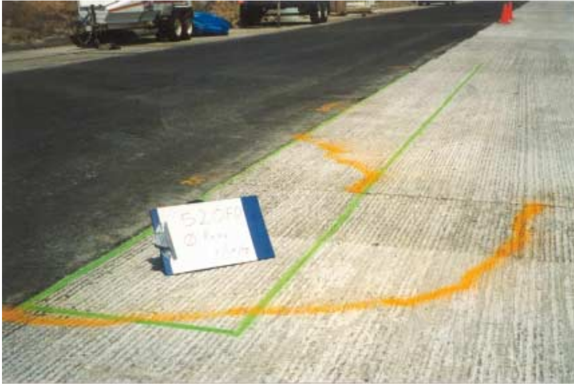
Photograph 4.8. Corner cracks at start of test, Test Section 520FD.
