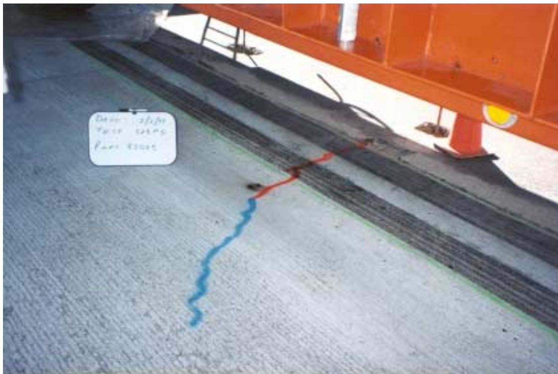
Photograph 4.35. Final crack pattern after 83,000 repetitions, Test Section 528FD.
