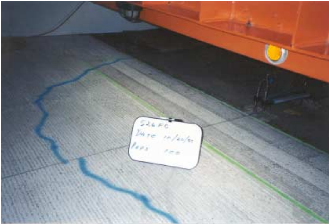
Photograph 4.28. Corner cracks after 100 repetitions, Test Section 526FD.
