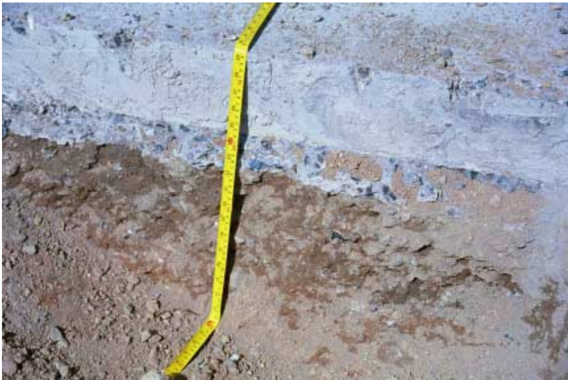
Photograph 5.4. Surface crack that did not propagate to bottom of concrete, Test Section 529FD.
