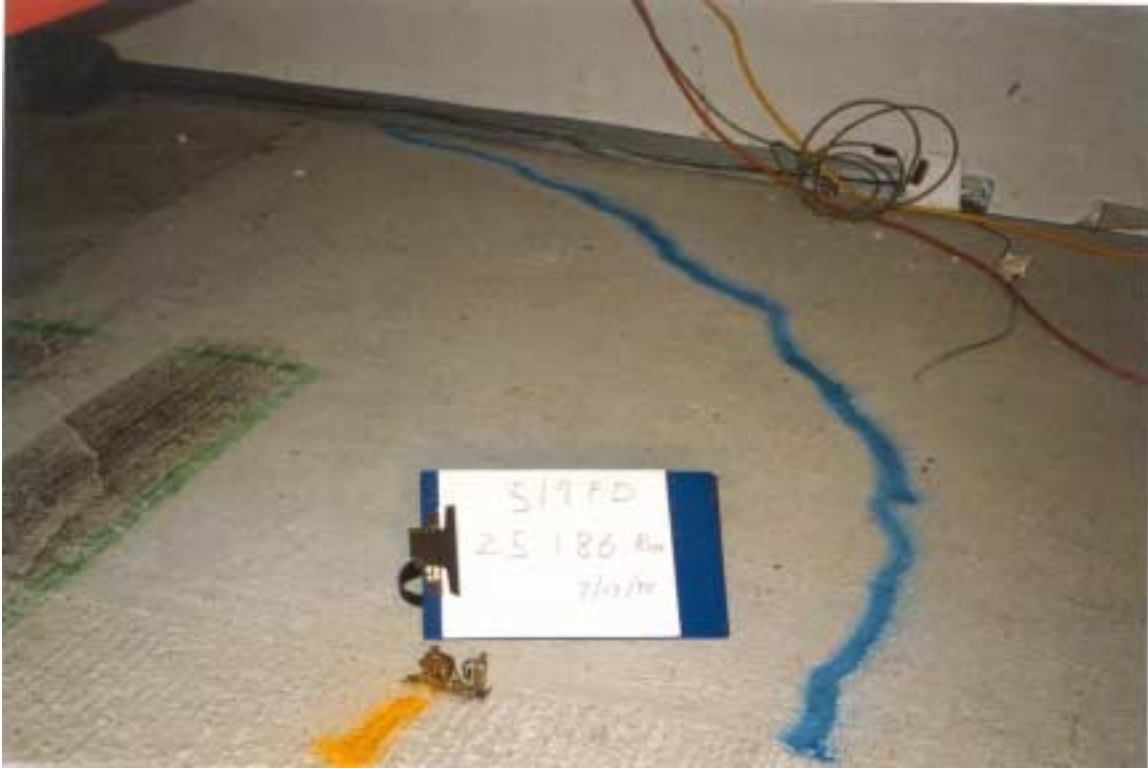
Photograph 4.3. Corner crack on slab 5 after 25,000 repetitions, Test Section 519FD.
