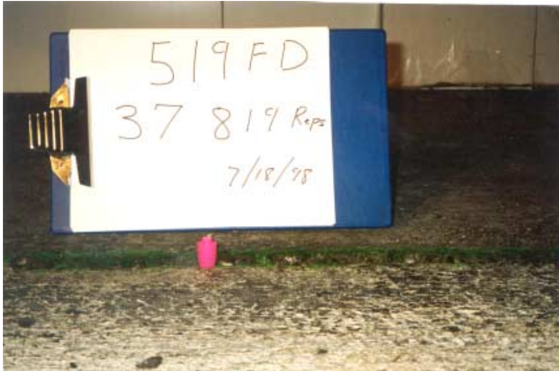
Photograph 4.6. Permanent deformation at shoulder after 37,000 repetitions, Test Section 519FD.
