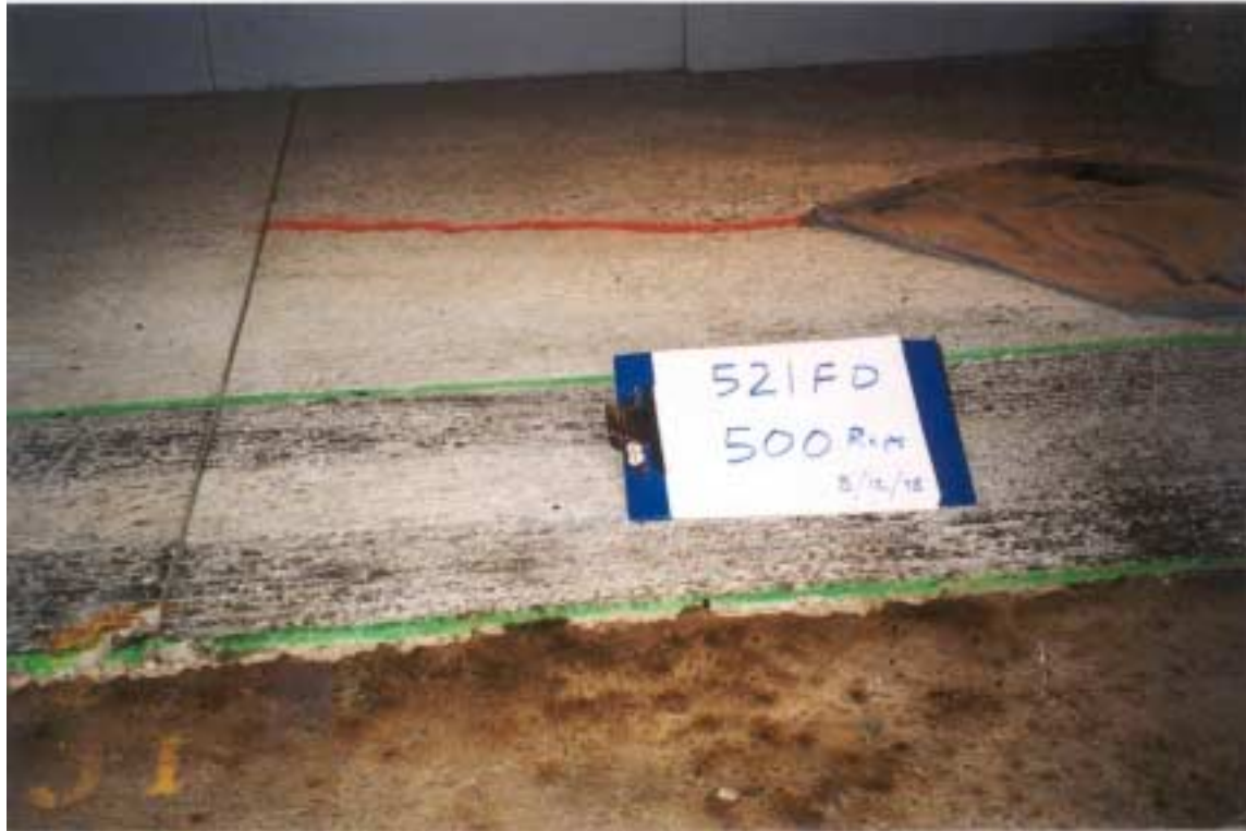
Photograph 4.14. Longitudinal crack on slab center after 500 repetitions, Test Section 521FD.
