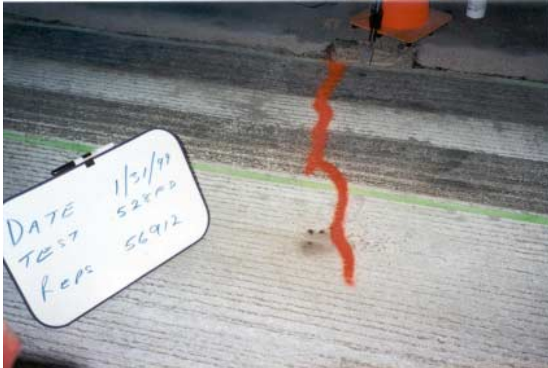
Photograph 4.34. Transverse crack after 52,000 repetitions, Test Section 528FD.
