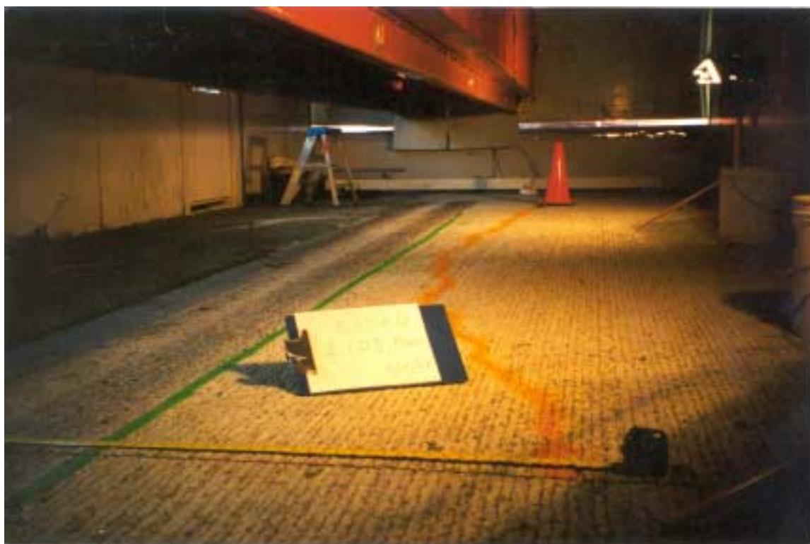
Photograph 4.2. Longitudinal crack after 2,105 repetitions, Test Section 519FD.
