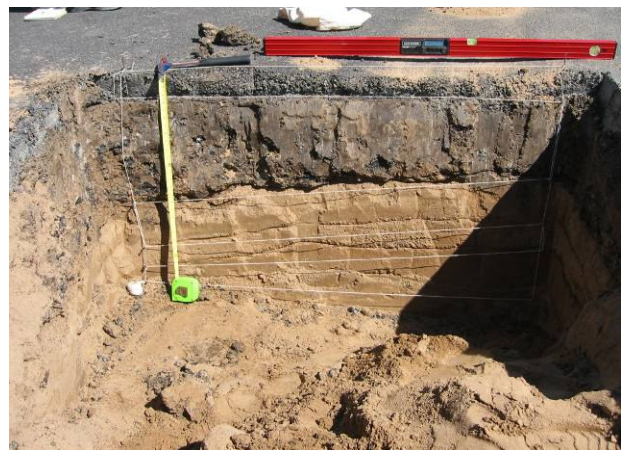
Layer differentiation with string lines
