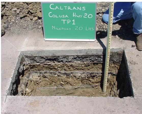
Layer differentiation with string lines
