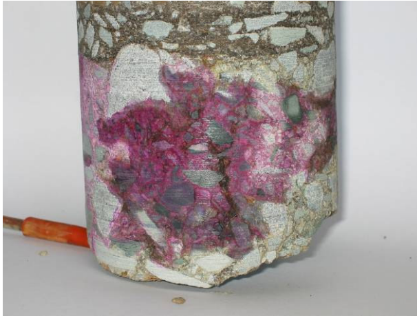
Phenolphthalein reaction on core
