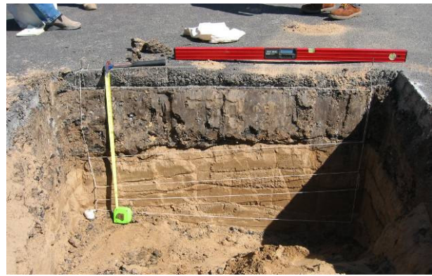
Note variable thickness of all layers.
