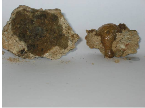
Hydrochloric acid reaction on disintegrated core
