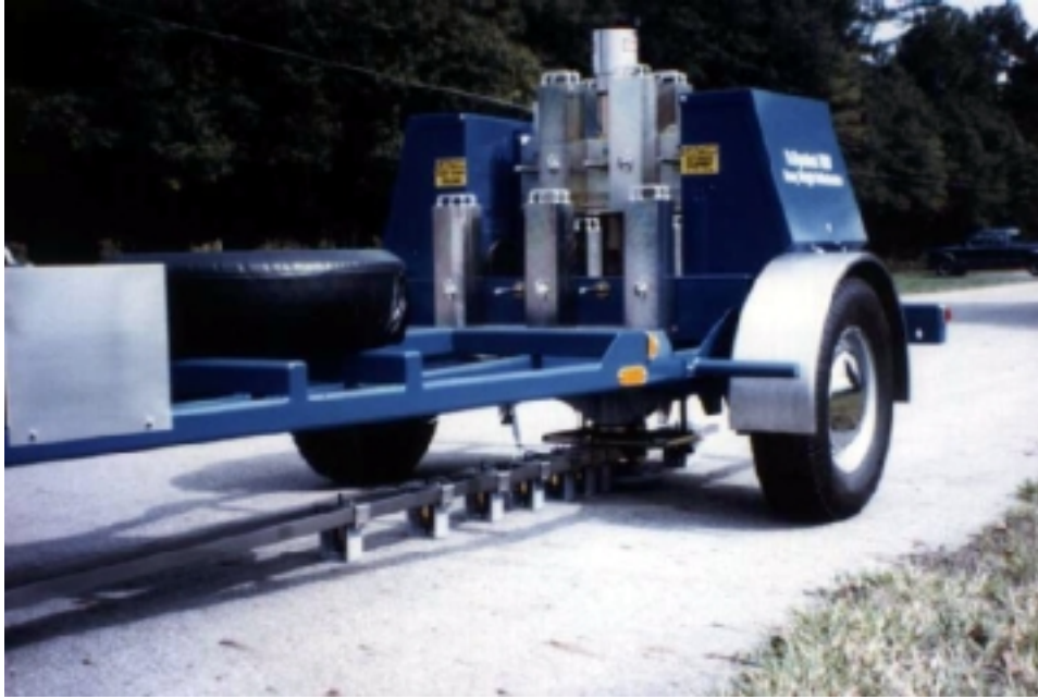
Figure 5. Heavy Weight Deflectometer.
