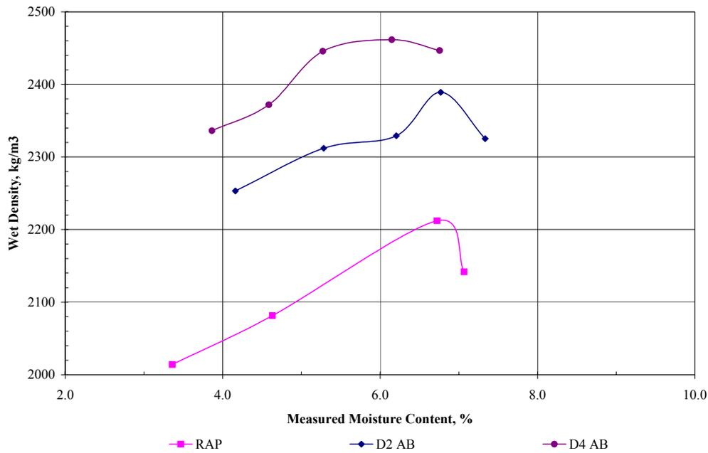
**Figure 12. Moisture density curves from CTM 216 performed on three base materials.**
