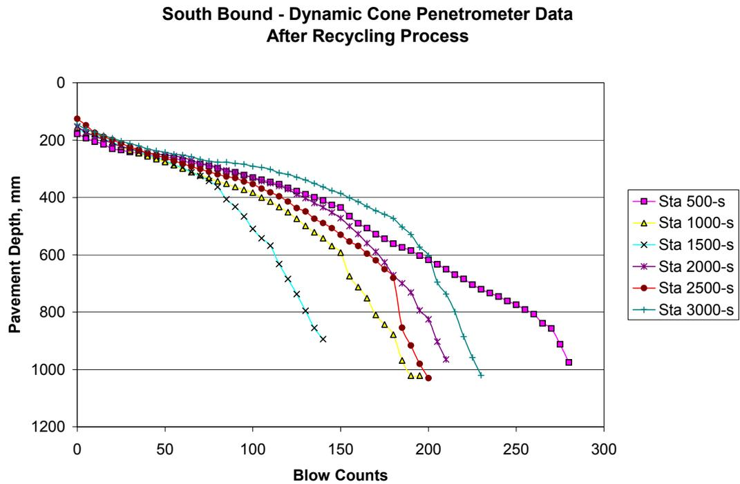
Figure 4. Typical DCP data from I-395.
