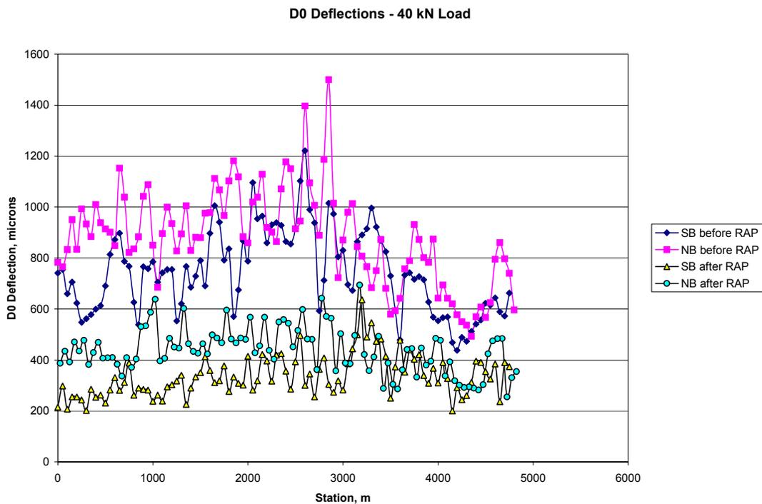
**Figure 8. D0 deflections normalized at a 40-kN load.**
