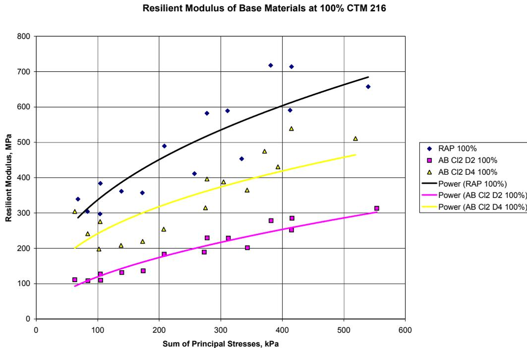
**Figure 17. Resilient modulus characteristics of base materials, 100 percent maximum wet density, CTM 216.**
