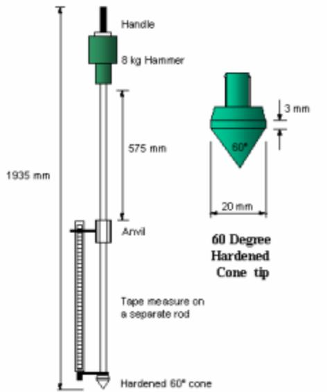
Figure 3. Schematic illustration of DCP device.
