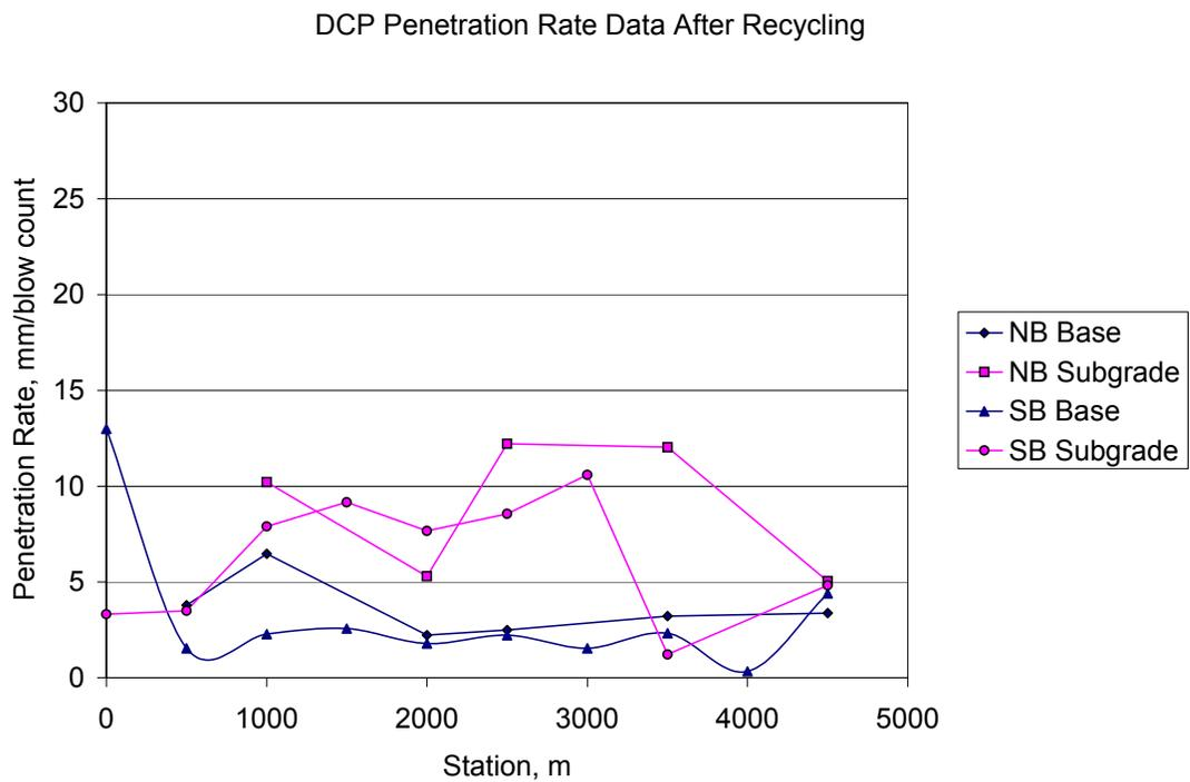
**Figure 6. DCP penetration rate after recycling process.**
