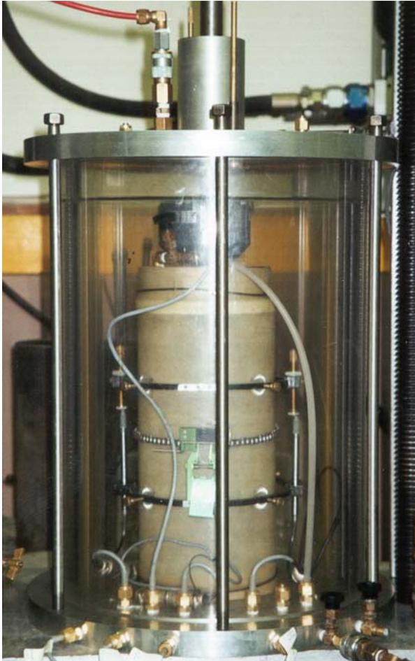
**Figure 13. University of California Berkeley Pavement Research Center triaxial testing system.**
