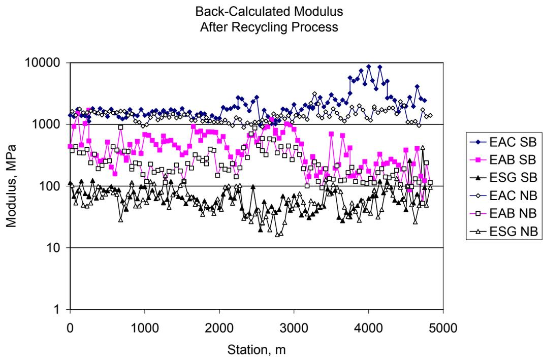
**Figure 10. Estimated moduli of pavement layers after recycling process.**
