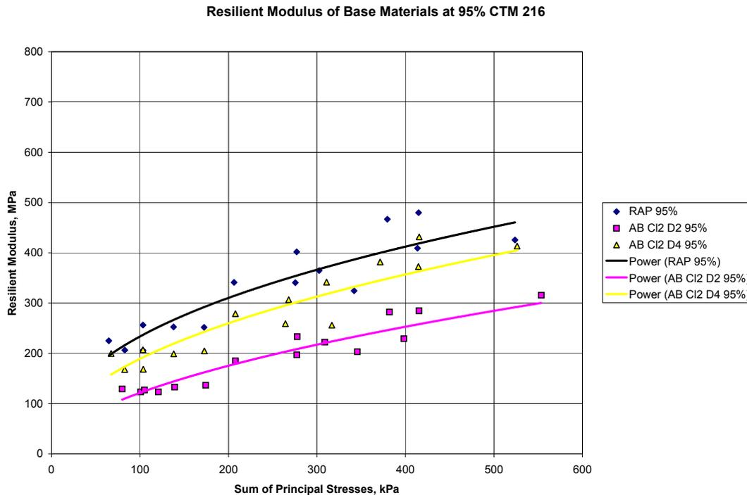
**Figure 16. Resilient modulus characteristics of base materials, 95 percent maximum wet density, CTM 216.**
