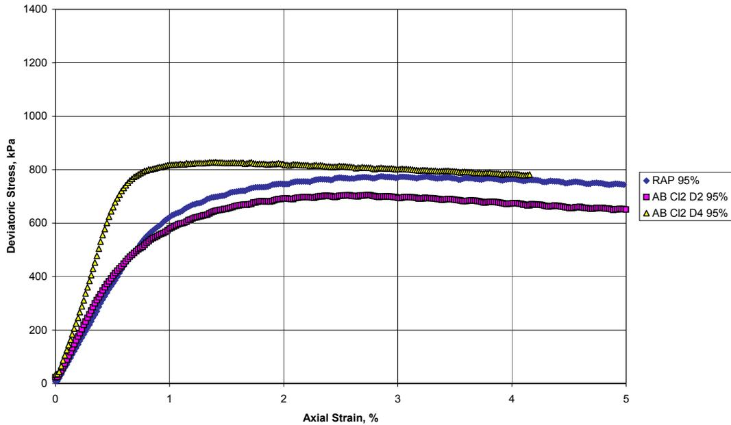
**Figure 14. Drained triaxial test CTM 216 performed at 95 percent maximum wet density and 105 kPa confining pressure.**
