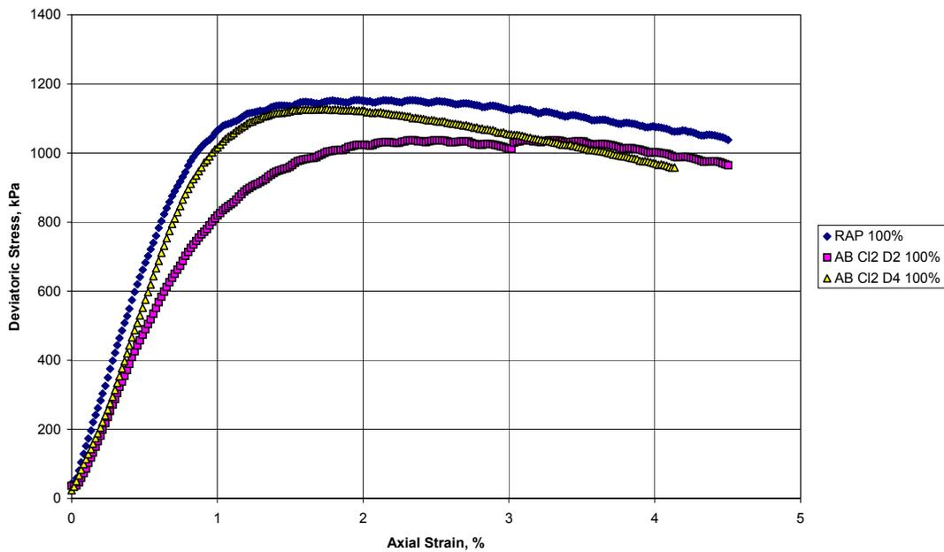
**Figure 15. Drained triaxial test CTM 216 performed at 100 percent maximum wet density and 105 kPa confining pressure.**
