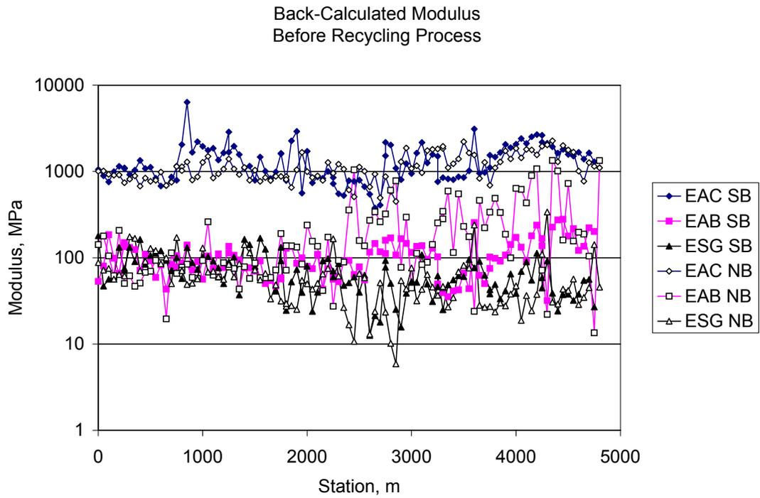
**Figure 9. Estimated moduli of pavement layers before recycling process.**
