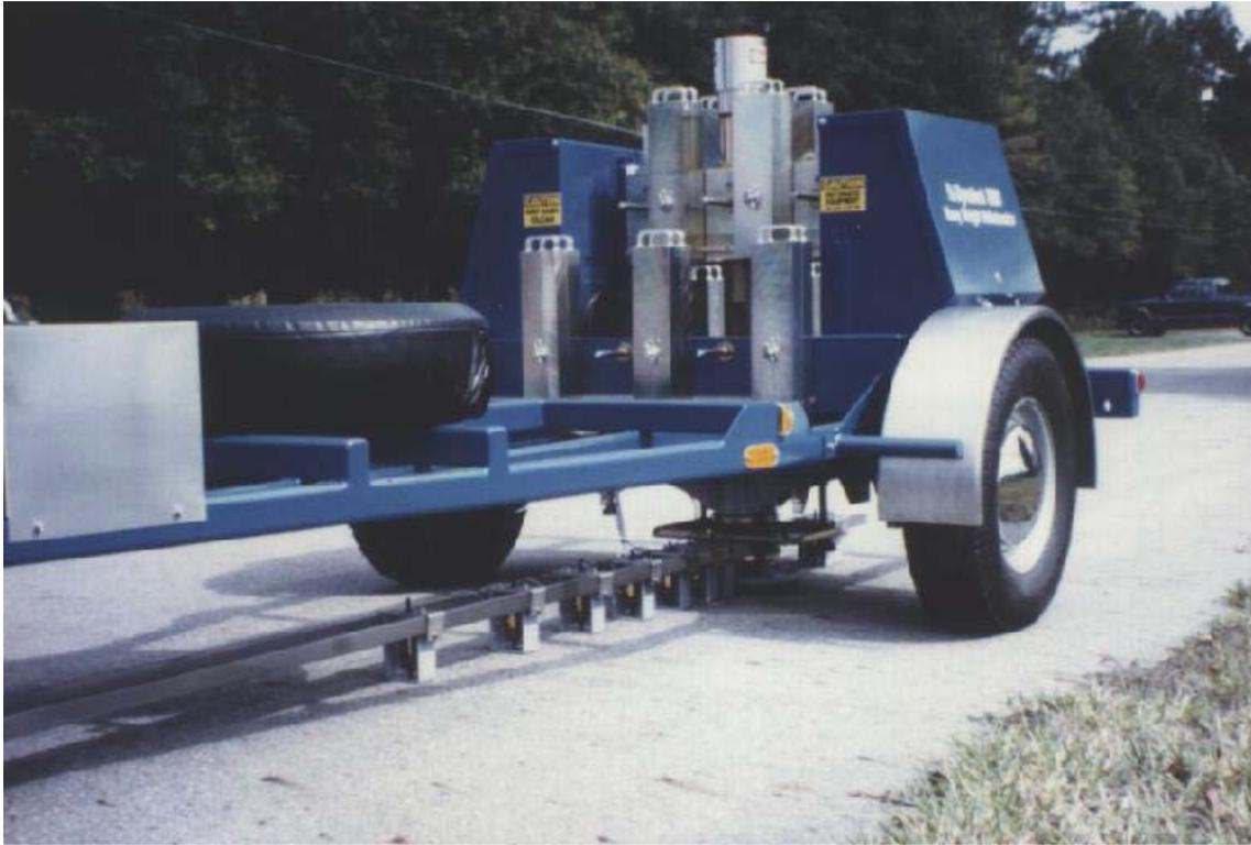
**Figure 7. Heavy Weight Deflectometer.**
