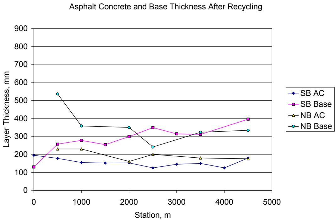
**Figure 2. Pavement thickness profile after recycling process.**
