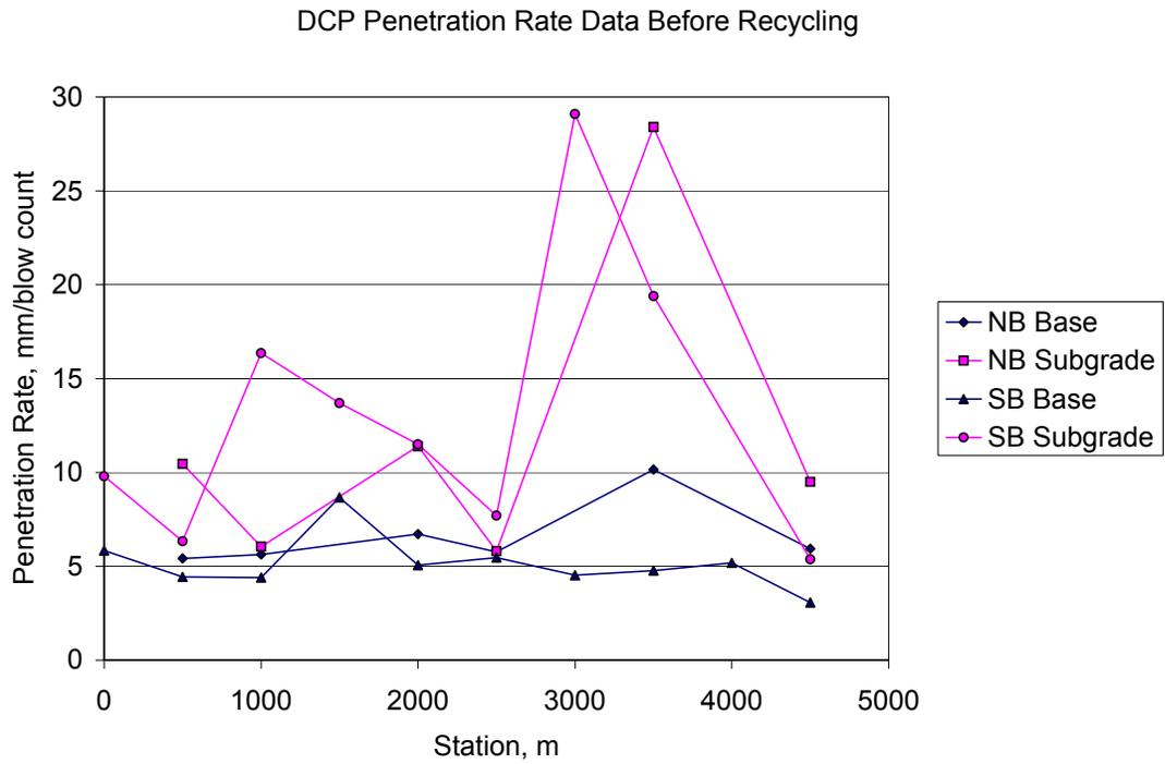
**Figure 5. DCP penetration rate before recycling process.**
