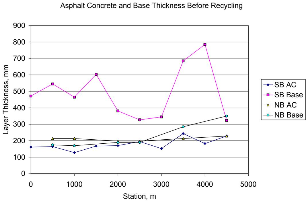
**Figure 1. Pavement thickness profile before recycling process.**
