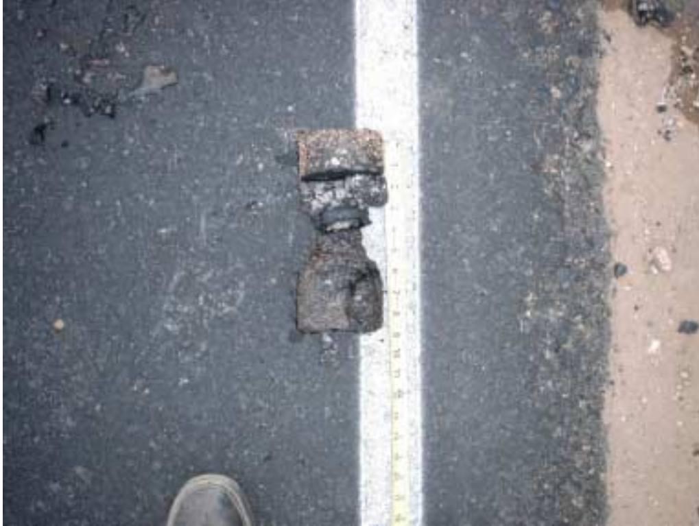
Figure C11. Core from westbound lane at station 152+00, showing evidence of stripping in middle AC layers.
