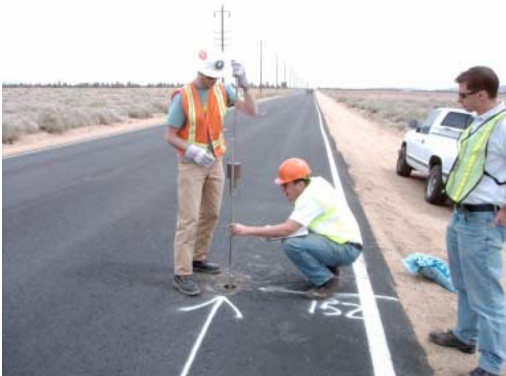
Figure C2. Dynamic Cone Penetrometer (DCP) operation at station 152+00 in March, 2002.
