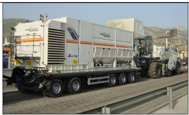
(b) Rotary mixer/recycler coupled to slurry applicator
