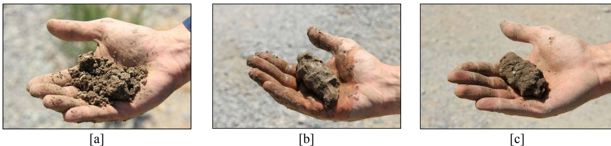
Figure 5.5: Squeeze test for assessing moisture content. ([a] too dry, [b] too wet, and [c] acceptable)
