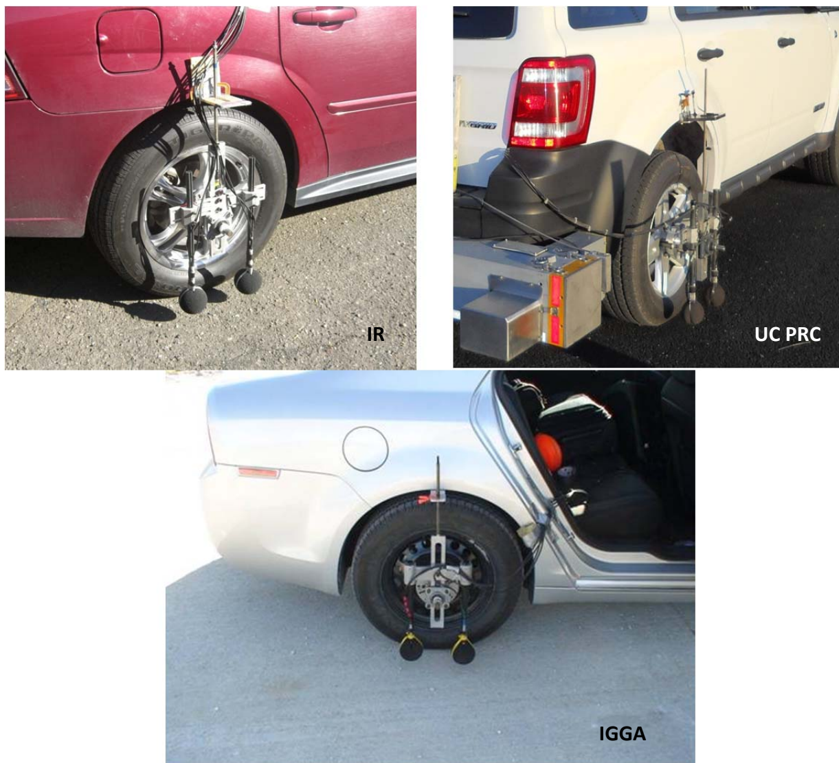
Figure 3: OBSI fixtures on IR, UC PRC, and IGGA test vehicle
