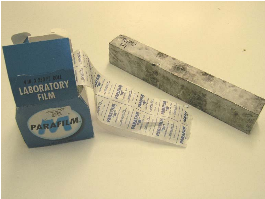
Figure 6-12. Fatigue beam specimen wrapped with Parafilm.
