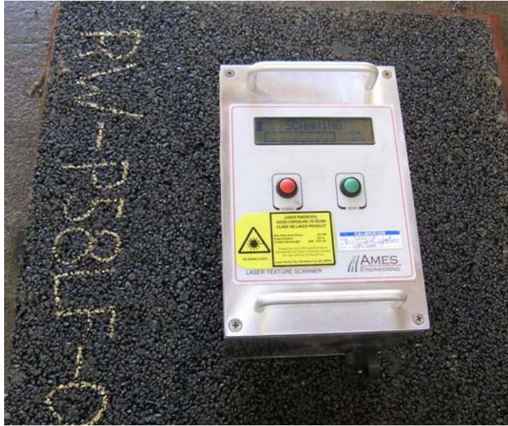
Figure 4.8: The AMES Engineering laser texture scanner.
