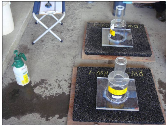
Figure 4.16: Permeability testing on compacted slabs.
