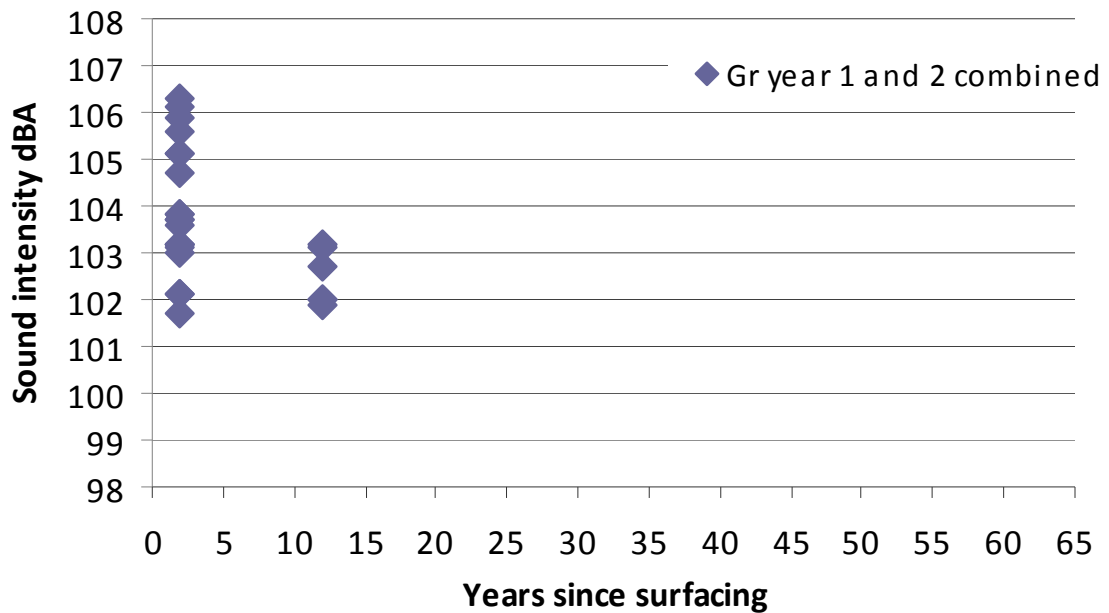
Figure 3.35: Year 1 and Year 2 OBSI values for all diamond grooved sections versus years since last surfacing.
