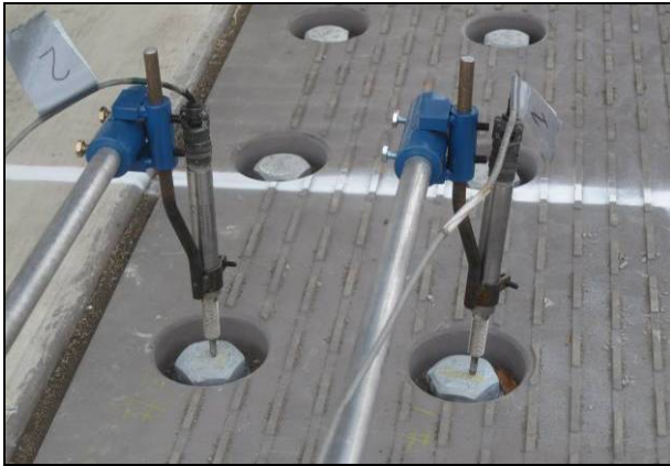
Figure 3.6: LVDTs on channel assembly bolts. (Instruments #1 and #2)
