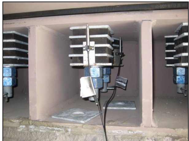
Figure 3.11: LVDT on bottom of steel plate. (Instrument #13)
