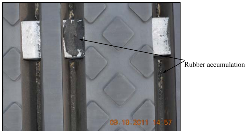
Figure 4.27: Phase 1.3: Rubber particle accumulation on Trelleborg unit after 740,000 repetitions.
