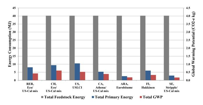
Figure 4.4: Bitumen production, at refinery (1 kg).
