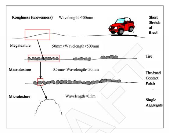
Figure 1.4: Pavement texture and wavelength (Sandberg, 1997, pp 3).
