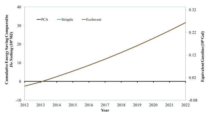
Figure B.17: Sensitivity analysis for data source of cumulative energy saving compared to *Do Nothing* with Type III cement using Smooth Rehab under 3% traffic growth rate in IMP-86.
