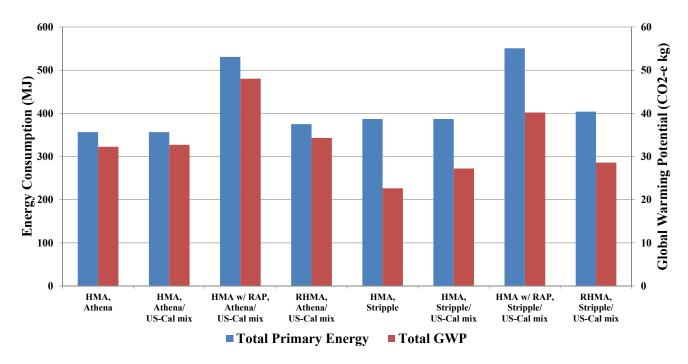
Figure 4.5: HMA mixing, at plant per metric tonne of asphalt mix produced. Note that one tonne of asphalt has a volume of approximately 0.36 to 0.5 m<sup>3</sup>.
