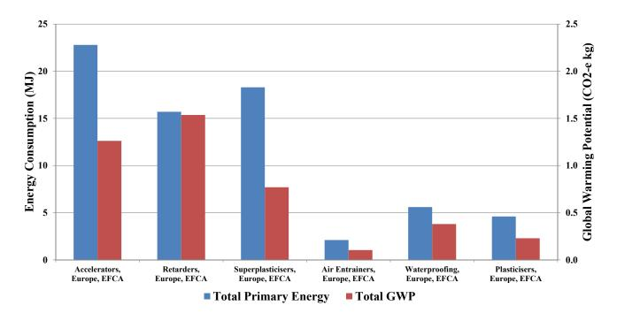
Figure 4.8: Concrete admixtures production, at plant (1 kg).
