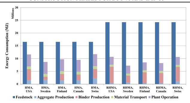
Figure C.1: BUT-70 Material Production Phase: energy consumption for the functional unit. Note: These are based on LCIs from five different regions. However, each LCI was updated and recalculated to reflect California conditions (i.e., the California-specific electricity mix).
