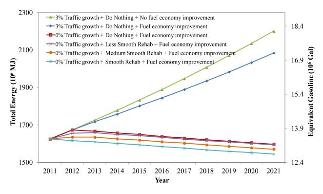
Figure 7.16: Energy consumption in Use Phase with 0 percent and 3 percent traffic growth on LA-5.
