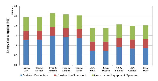
Figure C.5: IMP-86 Material Production Phase and Construction Phase: energy consumption for the functional unit.
