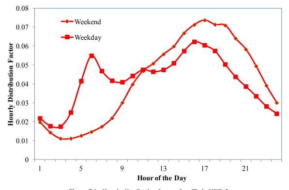
Figure 7.1: Hourly distribution factor of traffic in KER-5.
