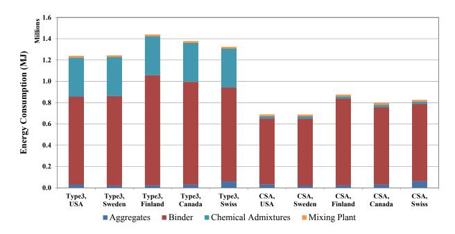
Figure C.7: IMP-86 details of Material Production Phase: energy consumption for the functional unit.
