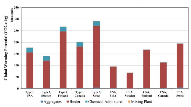
Figure C.8: IMP-86 details of Material Production Phase: GHG emissions (metric tons) for the functional unit.
