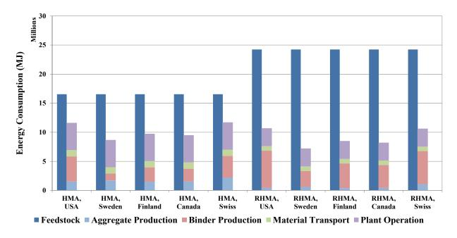
Figure 7.7: KER-5 Material Production Phase: energy consumption for the functional unit. Note: These are based on LCIs from five different regions. However, each LCI was updated and recalculated to reflect California conditions (i.e., the California-specific electricity mix).
