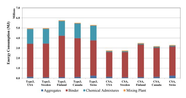
Figure 7.13: LA-5 Details of Material Production Phase: energy consumption for the functional unit.
