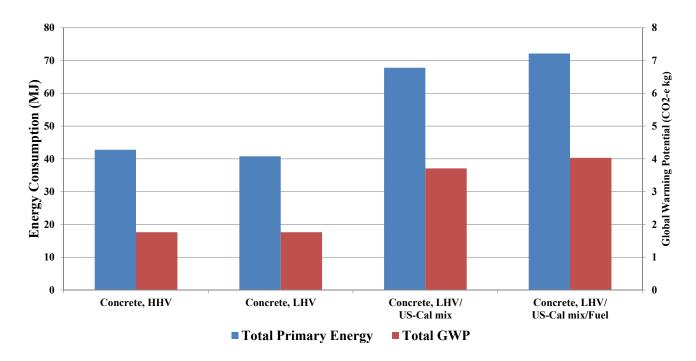
Figure 4.9: Concrete mixing, at plant, per 1 m<sup>3</sup> of concrete mix produced. (35) (Note that 1 m<sup>3</sup> of concrete has a mass of approximately 2.2 to 2.6 metric tonnes.)
