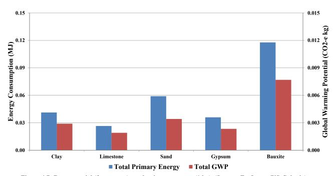
Figure 4.7: Raw material (for cement) production, at quarry (1 kg). (Source: EcoInvent/US-Cal mix)
