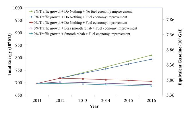
Figure 7.15: Energy consumption in Use Phase with 0 percent and 3 percent traffic growth on KER-5.
