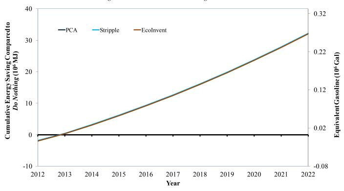
Figure B.18: Sensitivity analysis for data source of cumulative energy saving compared to *Do Nothing* with CSA cement overlay using *Smooth Rehab* under 3% traffic growth rate in IMP-86.
