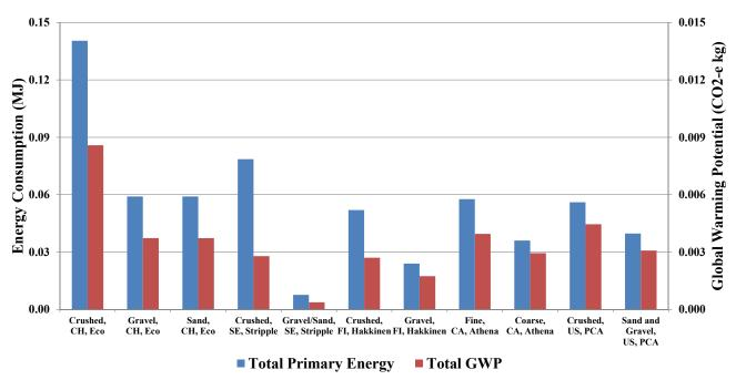
Figure 4.3: Aggregate production, at quarry (1 kg).
