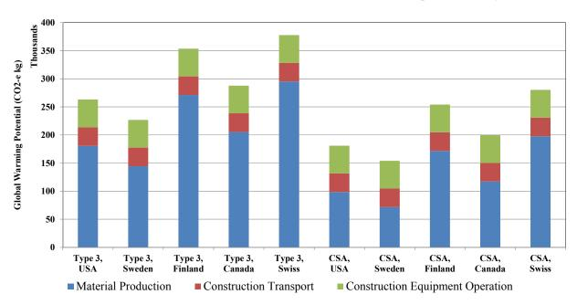
Figure C.6: LA-5 Material Production Phase and Construction Phase: GHG emissions for the functional unit (metric tons).
