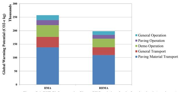
Figure C.4: BUT-70 Construction Phase: GHG emissions for the functional unit (metric tons).
