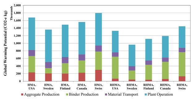
Figure 7.8: KER-5 Material Production Phase: GHG emissions for the functional unit (metric tons). Note: These are based on LCIs from five different regions. However, each LCI was updated and recalculated to reflect California conditions (i.e., the California-specific electricity mix).
