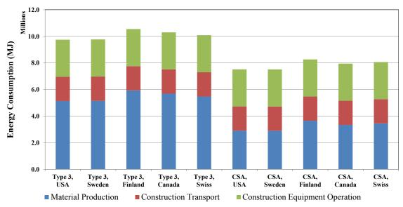
Figure 7.11: LA-5 Material Production Phase and Construction Phase: energy consumption for the functional unit.
