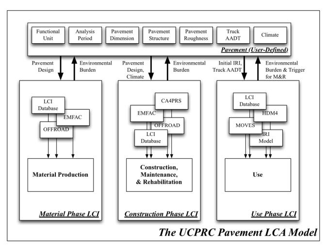
Figure 3.2: Overview of UCPRC Pavement LCA model.
