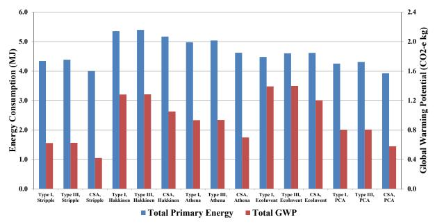
Figure 4.6: Cement production, at plant (1 kg), for Type I cement and estimated for Type III and CSA based on Type I LCI.
