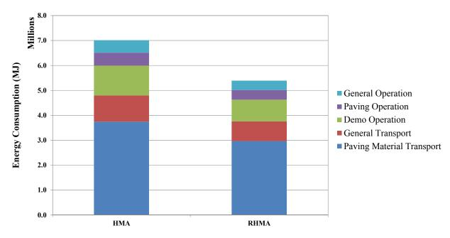
Figure 7.9: KER-5 Construction Phase: energy consumption for the functional unit.
