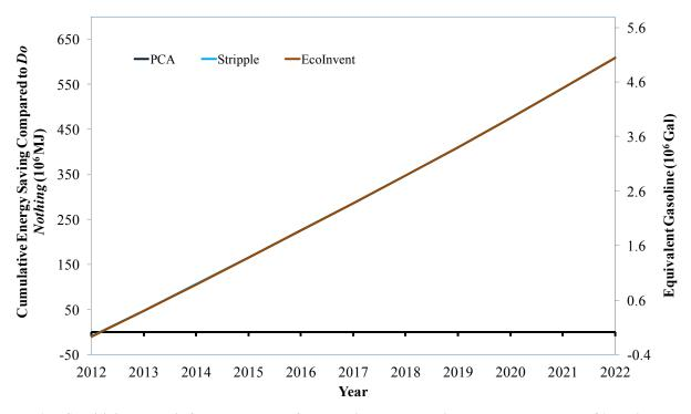
Figure B.15: Sensitivity analysis for data source of cumulative energy saving compared to *Do Nothing* with Type III cement using *Smooth Rehab* under 3% traffic growth rate in LA-5.
