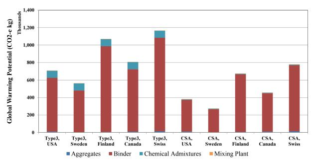
Figure 7.14: LA-5 Details of Material Production Phase: GHG emissions for the functional unit (metric tons).
