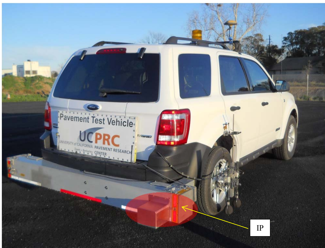
Figure 4.7: Instrumented vehicle with an inertial profiler (IP).
