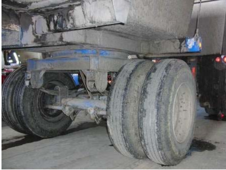
Figure 3.4: Company A trailer suspension.
