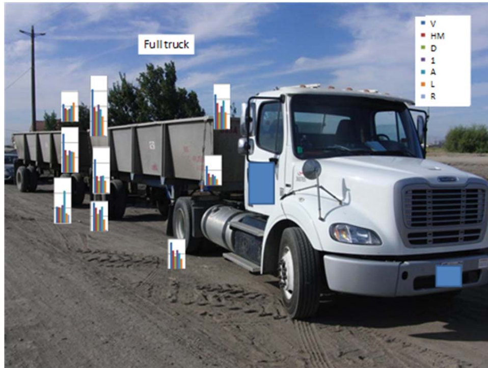
Figure 3.13: Typical accelerometer outputs—Company A, full truck.
