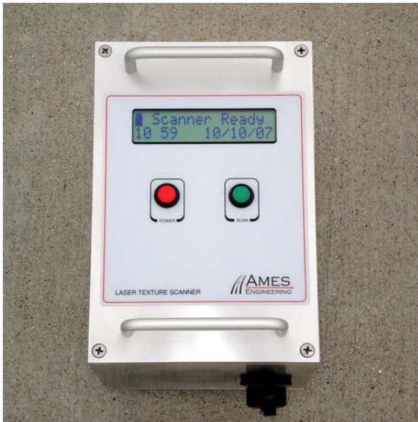
Figure 3.2: Laser texture scanner and an example of surface texture profile it measured (Section QP-158 with longitudinally tined texture). (Photo of LTS courtesy of Ames Engineering, Inc.)
