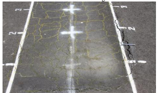
Cracking and deformation at end of test section
