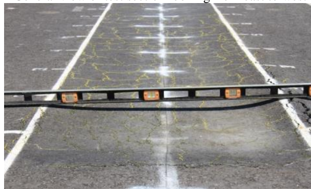
Cracking and deformation at end of test section
