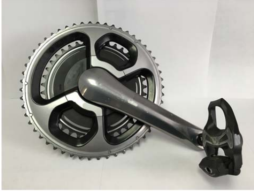
Figure 3.15: Manufacturer A power meter crank, front.
