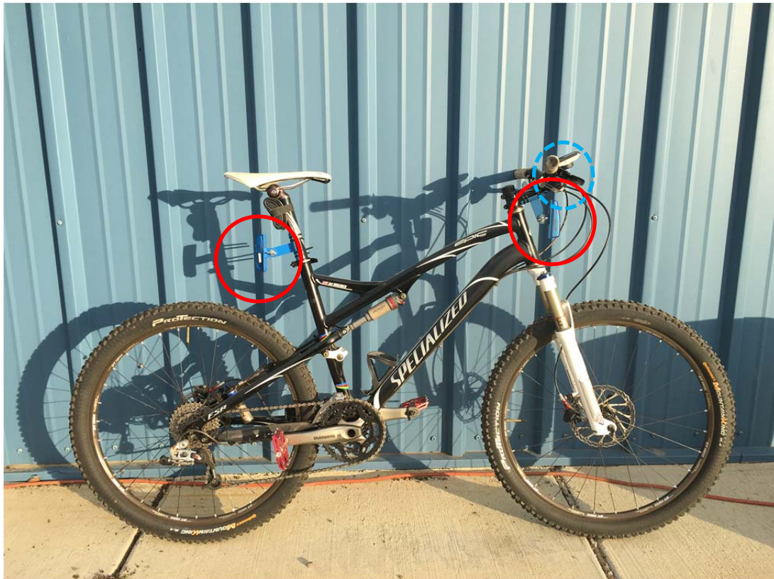
Figure 3.8: Mountain bicycle instrumented with accelerometers (solid red circles) at the typical mounting locations and a GPS unit on the handlebar (circle of blue dashes).
