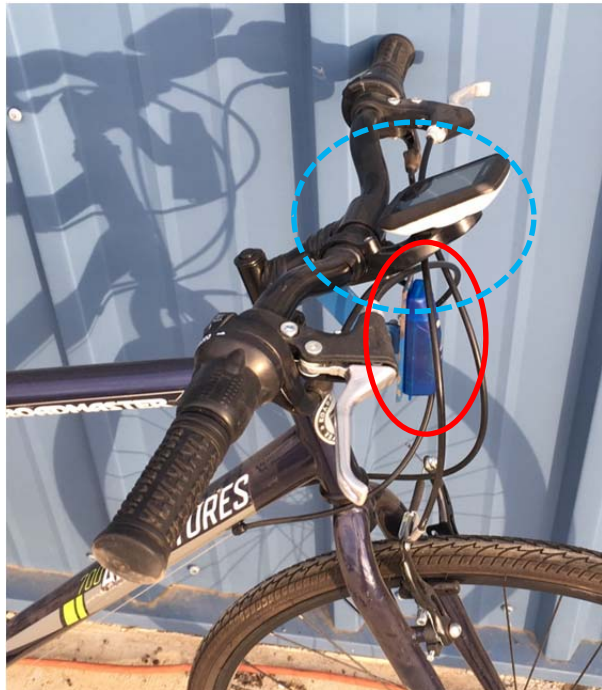
Figure 3.6: Detail of front of commuter bicycle instrumented with accelerometer (solid red circle) at the stem mounting location and a GPS unit on the handlebar (circle of blue dashes).
