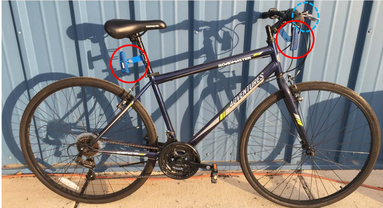
Figure 3.5: Commuter bicycle instrumented with accelerometers (solid red circles) at the typical mounting locations and a GPS unit on the handlebar (circle of blue dashes).
