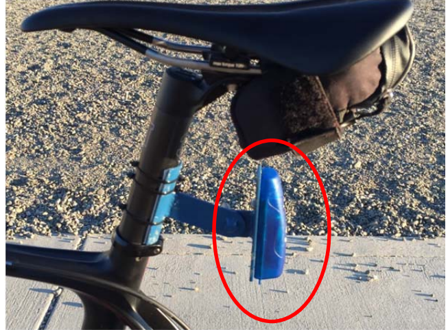
Figure 3.4: Detail of rear of road bicycle instrumented with accelerometer (solid red circle) at the seatpost mounting location.
