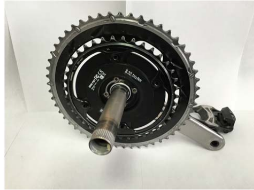
Figure 3.16: Manufacturer A power meter crank, rear.
