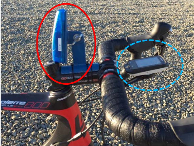
Figure 3.3: Detail of front of road bicycle instrumented with accelerometer (solid red circle) at the stem mounting location and a GPS unit on the handlebar (circle of blue dashes).
