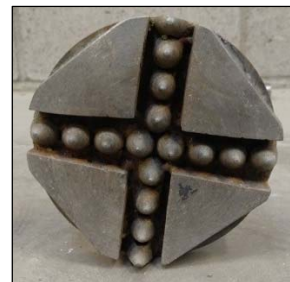
Figure 6.5: Scouring tool: general view and bottom view.
