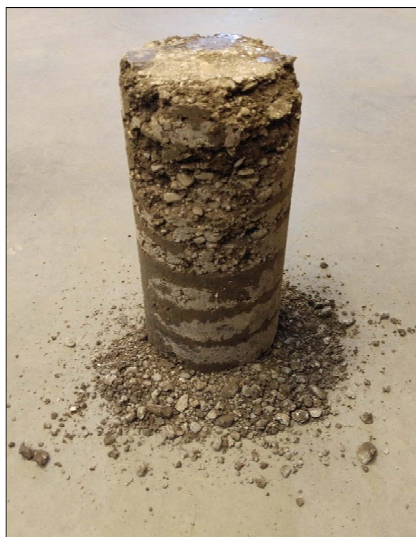
Figure 5.2: Result of microcracking effort with vibrating hammer.
