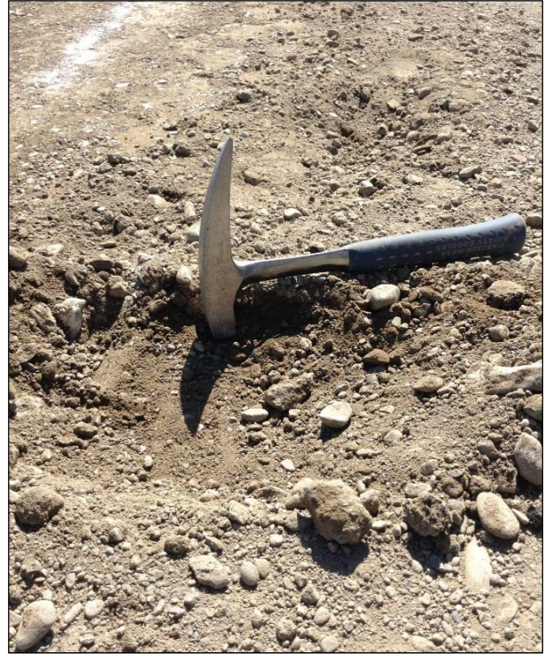
Figure 3.14: CR99: Depth of delaminated material (50 mm [2 in.]).
