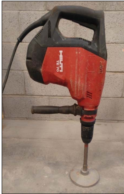
Figure 6.4: Vibrating compaction hammer with 148 mm compaction attachment.
