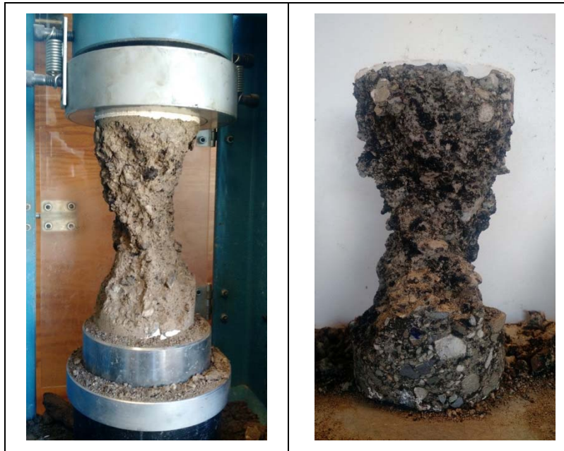
Figure 2.18: Shear failure of FDR-PC and FDR-FA specimens after UCS testing.
