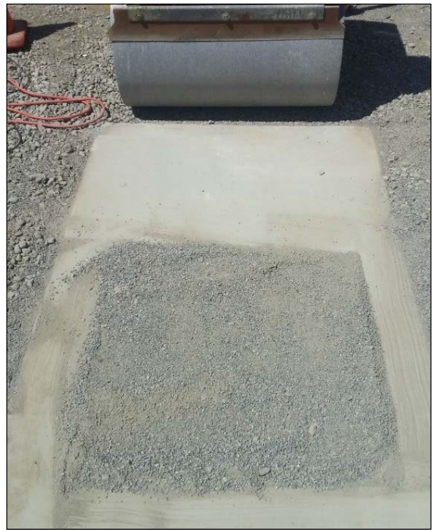
Figure 5.6: Final setup before microcracking.
