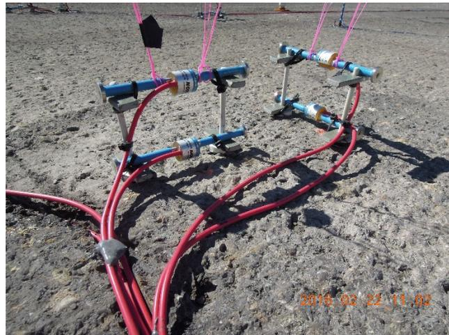
**Figure 2.4: Vibrating wire strain gages (VWSGs).**
