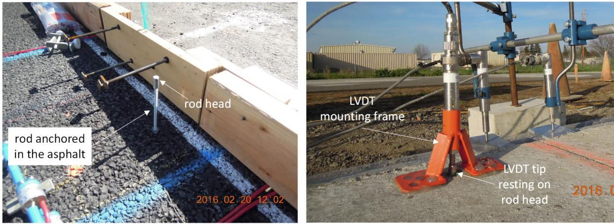
**Figure 2.9: Interface opening measuring device (IOMD).**
