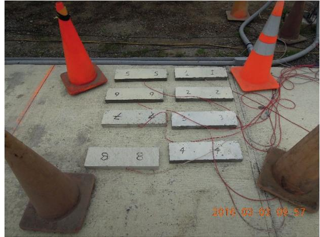
**Beams after demolding**
