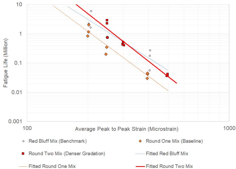
Figure 5.7: Comparison of the fatigue life of the Round One, Round Two, and Red Bluff mixes.
