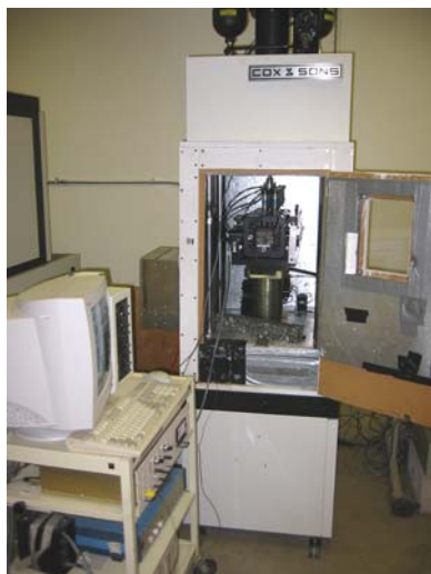
Figure 5: Moisture conditioning and flexural fatigue test equipment.
