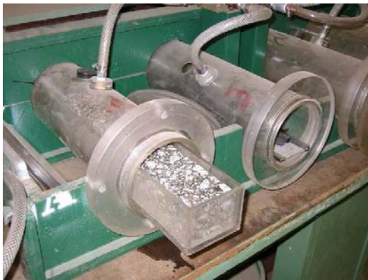
(a) Beam vacuum saturation equipment.
