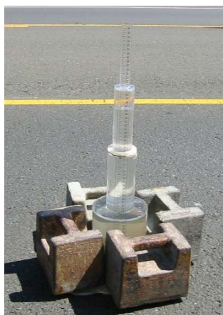
Figure 2: Falling-head permeameter used in the field.
