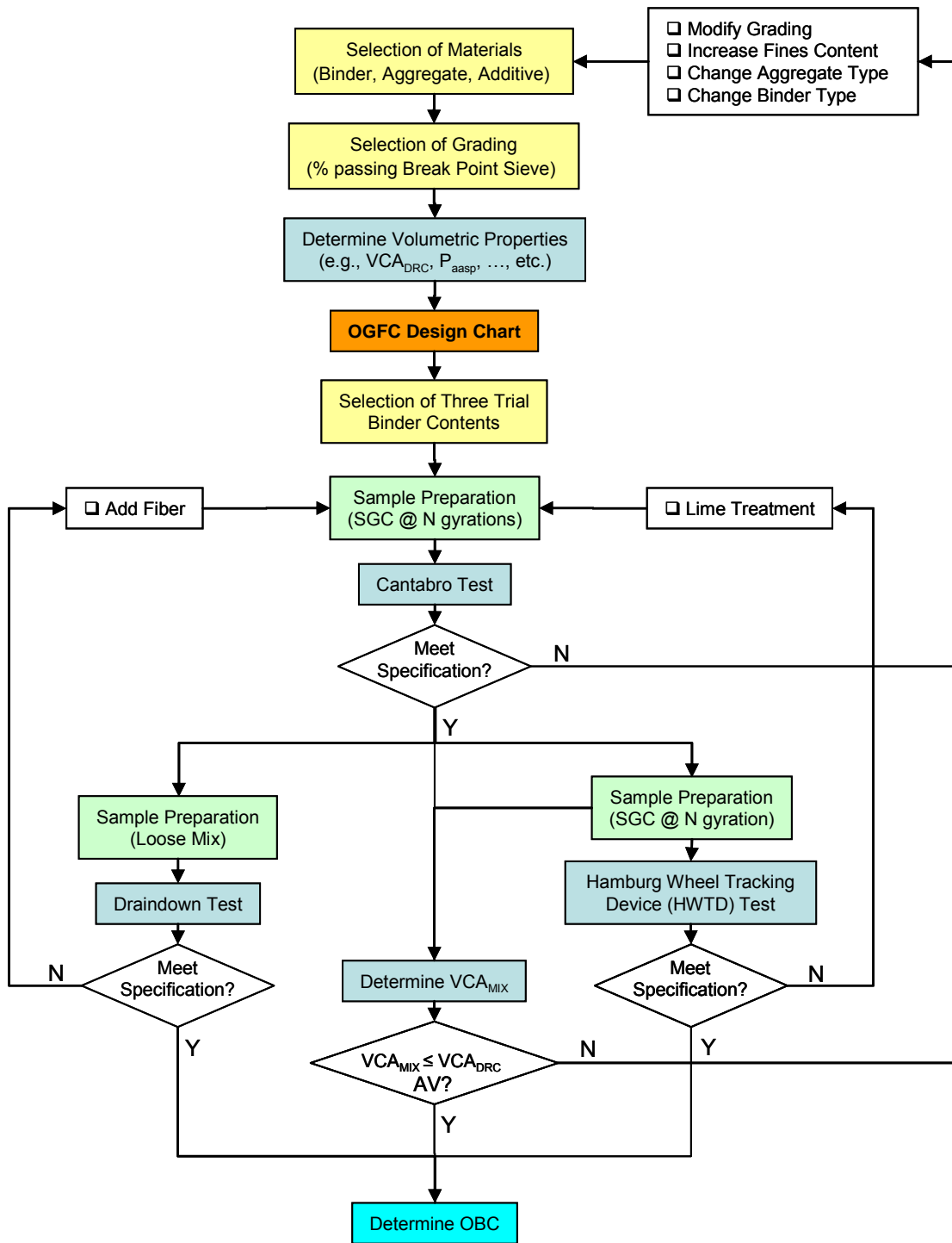
Figure 6.9: Proposed OGFC mix design procedure.
