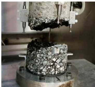
Tensile Testing of Composite Specimen. The composite specimens with new RHMA-G tended to fail in the asphalt rather than at the interface.
