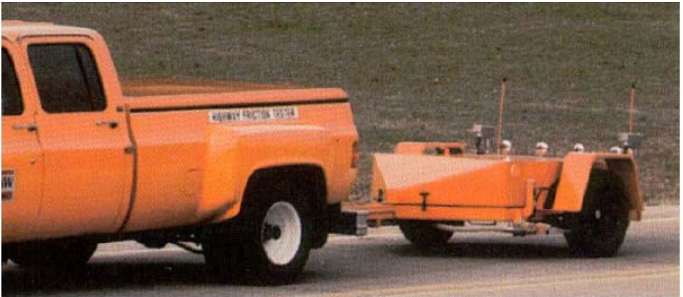
Figure 6: A typical ASTM standard skid trailer. (19)
