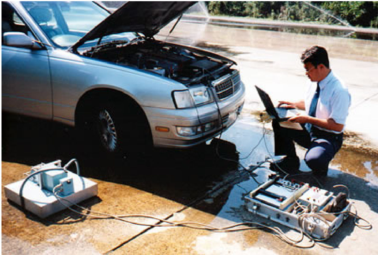
Figure 9: A Dynamic Friction Tester. (21)
