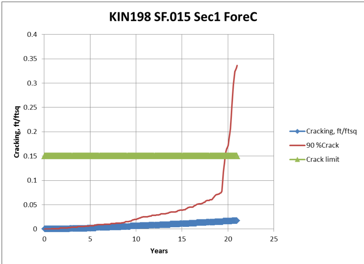
Figure A.9: Cracking-versus-time plot from CalME for a 0.10 ft (30 mm) RHMA-G overlay on Section 1. Note: The mean estimate of cracking after 20 years, with 50% reliability (0.02 ft/ft 2 ), is well below the failure criteria of 0.15 ft/ft 2 . After 18 years, there is a 90% reliability of cracking not exceeding 0.08 ft/ft 2 . But after 20 years, cracking exceeding 0.15 ft/ft 2 can be expected.
