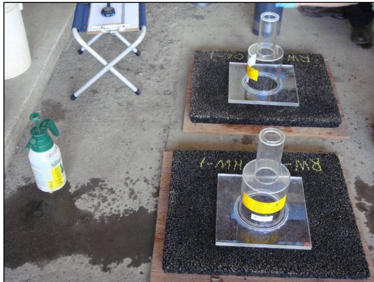
**Figure 7.1: Permeability testing on compacted slabs.**
