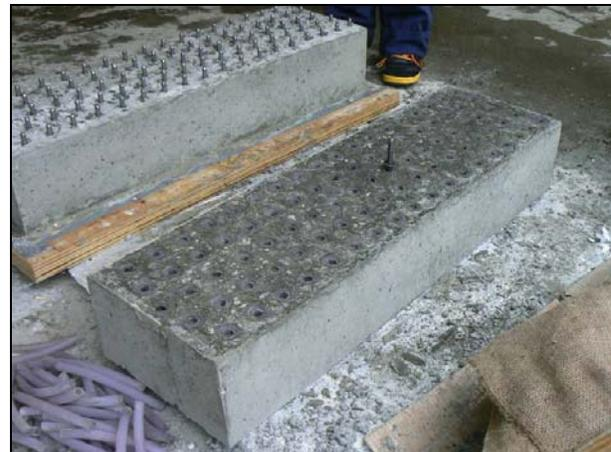
Figure 6.8: Demolded precast beam specimen.
