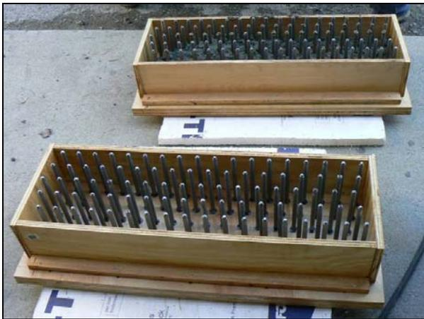
Figure 6.7: Precast beam specimen molds.
