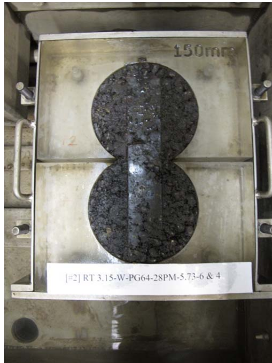
Figure C.1: HWTT result for PG 64-28PM 15% RAP, 1.2% lime (set #1, rt.) after 40,000 passes.
