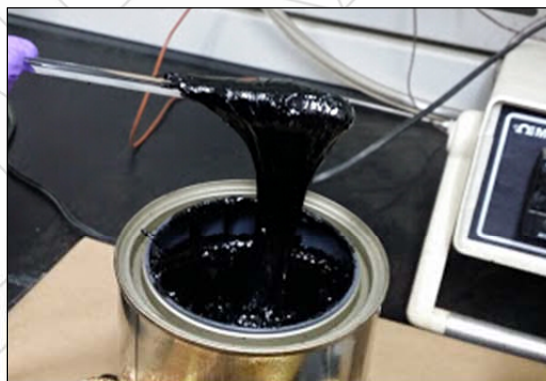
Figure 3.1: Recovered RAS binder after three hours of conditioning at 190°C.
