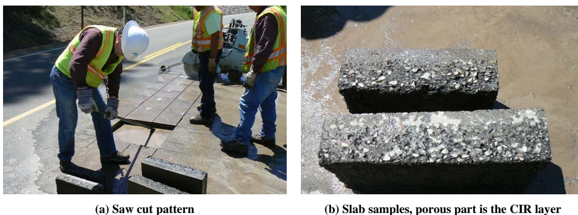
Figure 3.1: Taking slabs from the field to produce beam and core specimens in the laboratory
