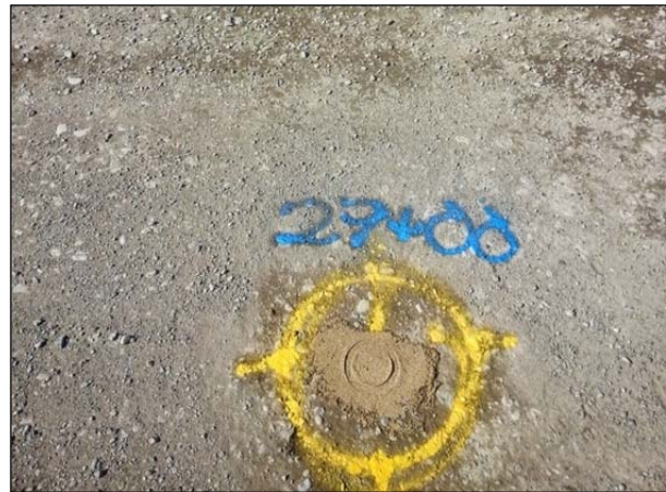
Figure 3.4: SSG footprint in sand patch.
