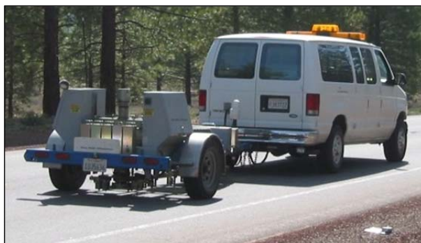
Figure 3.1: Falling weight deflectometer.
