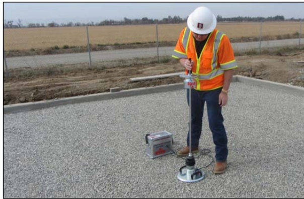
Figure 3.2: Light weight deflectometer.
