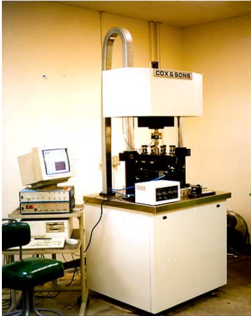
Figure 3.1. Conventional fatigue testing machine.
