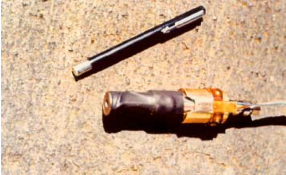
Figure 2.8. LVDT module of MDD (after CSIR).
