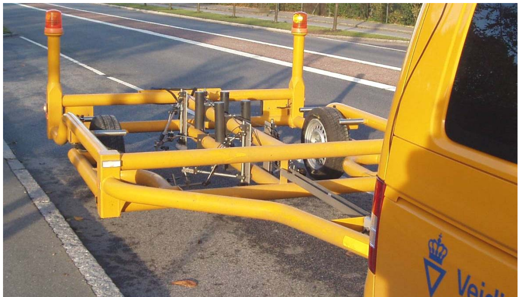
Figure 6.5. The CPX-trailer "deciBella" operated by the Danish Road Directorate/Danish Road Institute.
