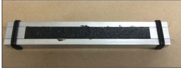
Figure 5.2: Prototype BBR mold for testing asphalt rubber binder.
