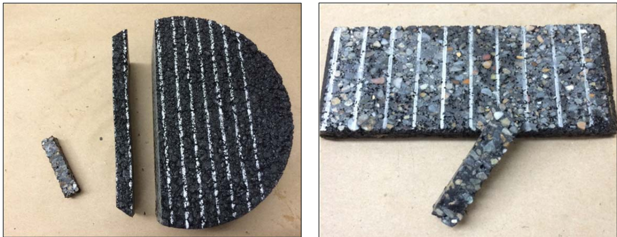
Figure 4.2: Cut FAM mix specimens (asphalt rubber binder).
