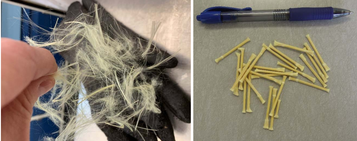
Figure 2.1: Aramid fibers (left) and fiber bundles (right).
