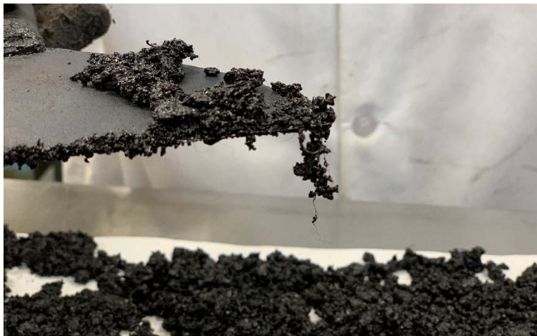
Figure 2.2: Asphalt mix reinforced with aramid fibers.
