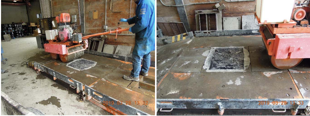
Figure 2.4: Rolling wheel compaction.
