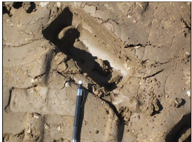
Figure 2.9: Breaking up of clay clods.
