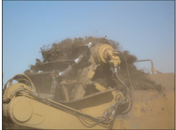
Figure 2.9: Breaking up of clay clods.
