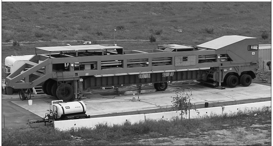
FIGURE 2 Heavy Vehicle Simulator (HVS)
