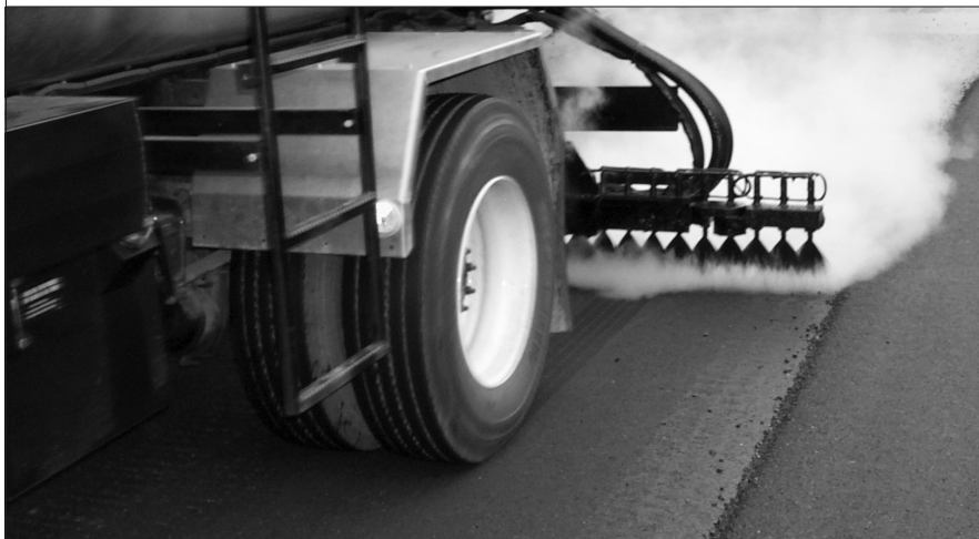
FIGURE 11 Proper overlap and spray bar height
