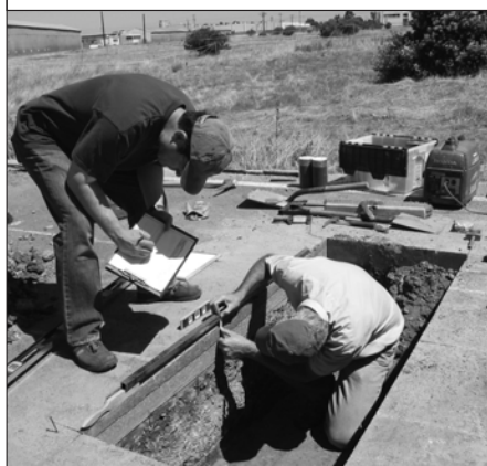
FIGURE 5 Forensic investigation of rutting in HVS test sections
