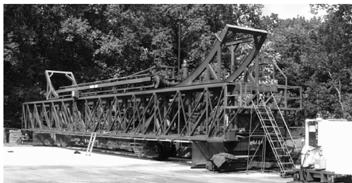
FIGURE 7 ALF testing device and close-up of loading wheel
