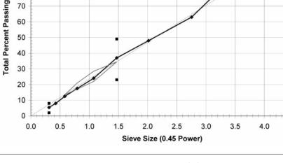
FIGURE 3 Aggregate Gradation Used on I-710 Long-Life Pavement Project
